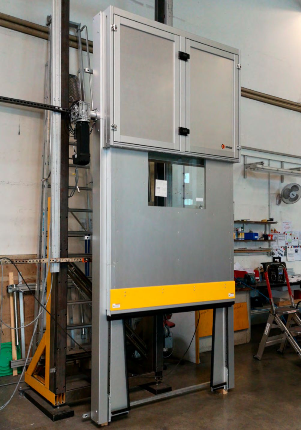
MecLock vertical safety window SFV.F-B99-E-7200-FO – servo-electric actuator sound insulated for engine test bench
