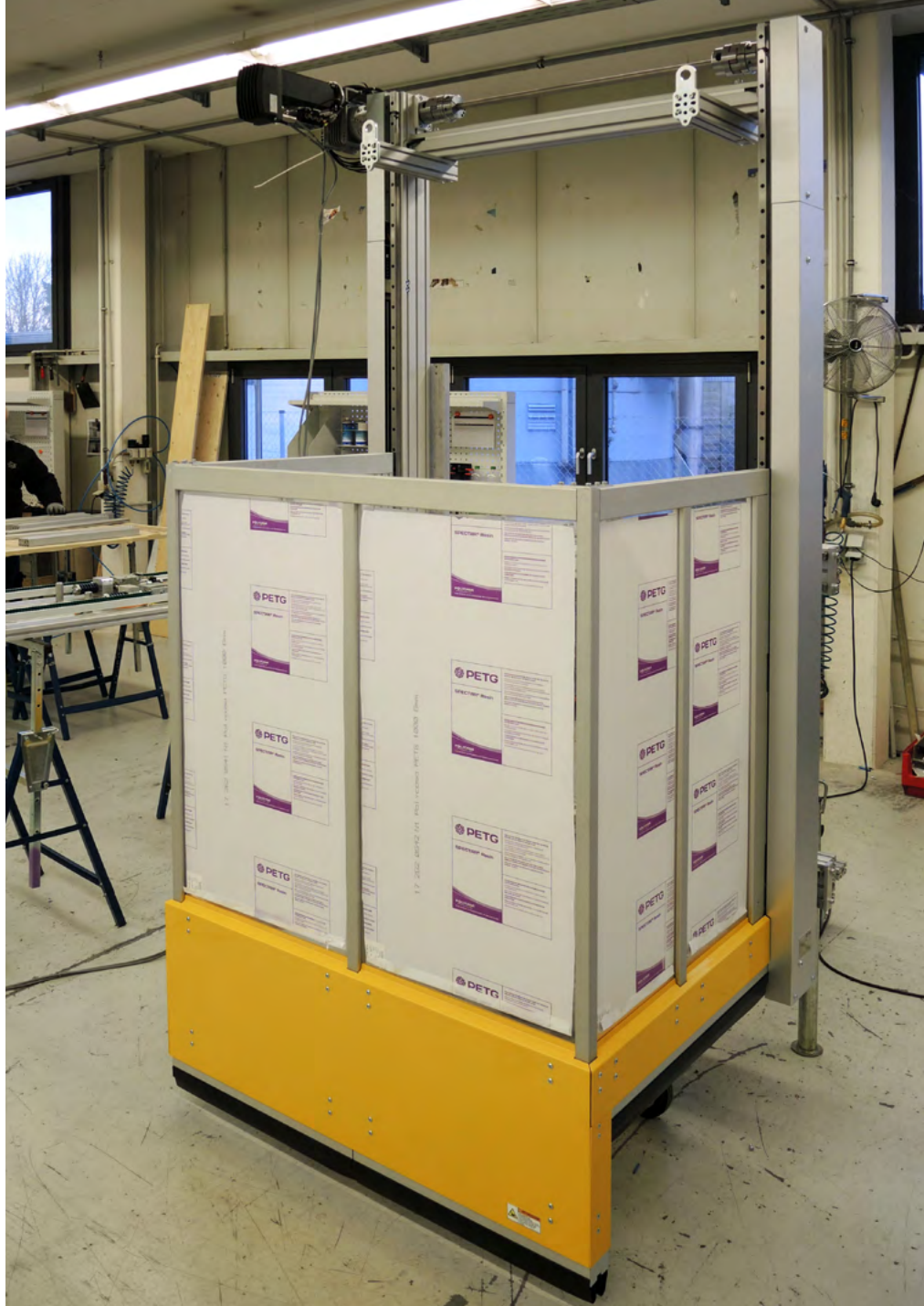
MecLock vertical safety window SFV.F-B30-E-7200-FO – servo-electric actuator protective field in U-shape – for medium and large protection areas – without upper panel protective field with contoured contact strips
