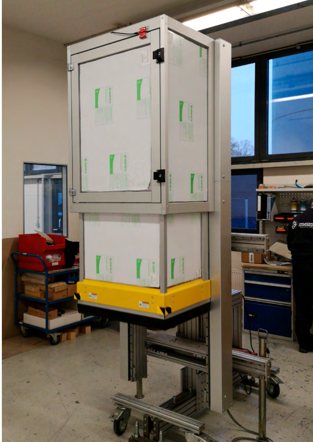
MecLock vertical safety window SFV.F-B30-E-7200-FO – servo-electric actuator protective field in U-shape for medium and large protection areas – panel with swing door closed penal door – intermediate position half stroke
