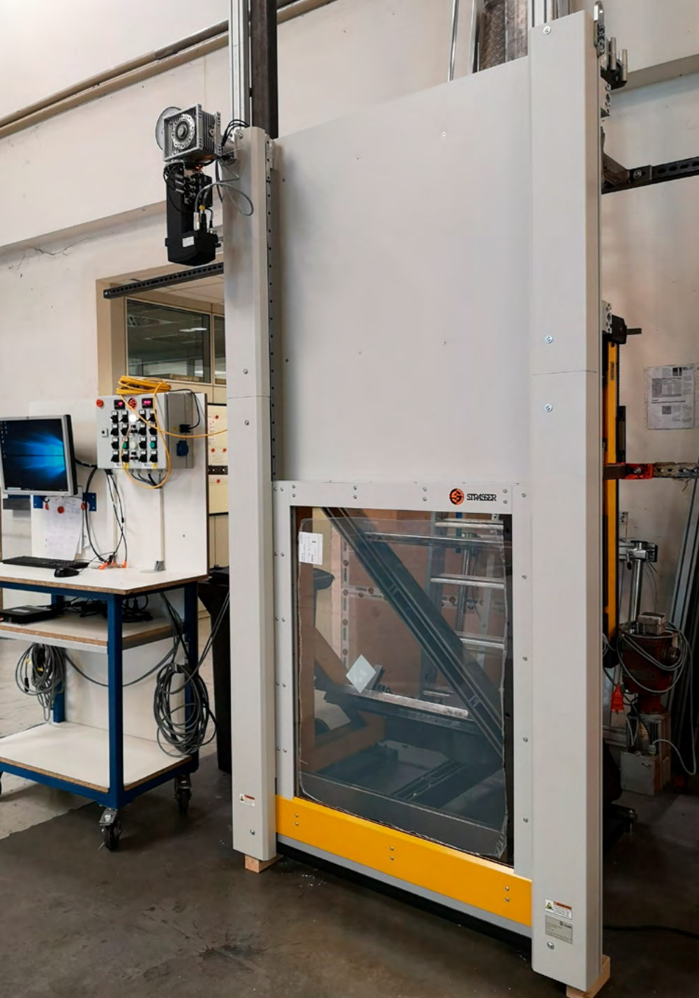
MecLock vertical safety window SFV.F-B99-E-7200-FO – servo-electric actuator for hydraulic test bench – reinforced pane frame with bulletproof glass 25 mm
