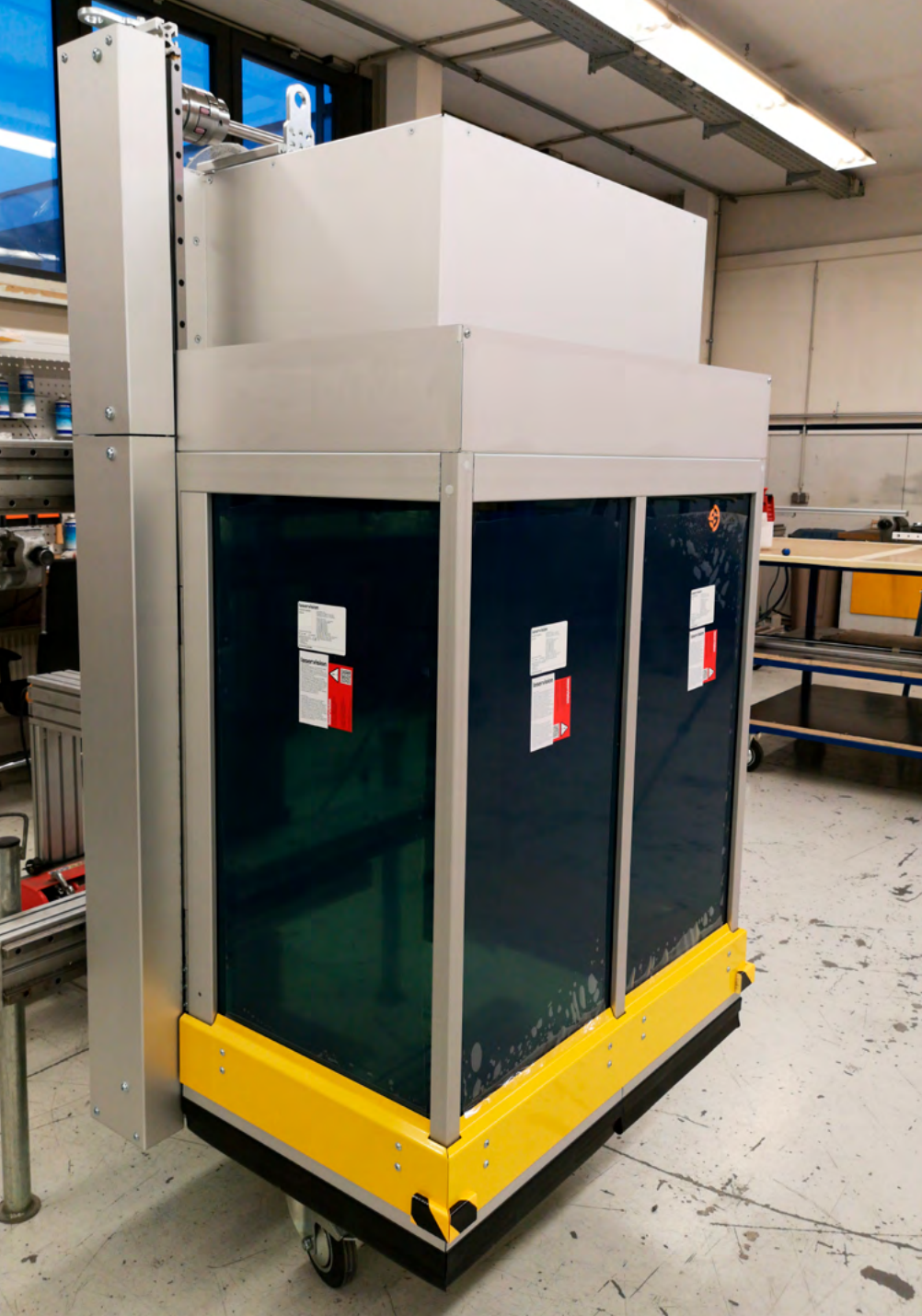
MecLock vertical safety window SFV.F-B99-E-7200-FO – servo-electric actuator protective field in U-shape for medium and large protection areas light-protected in labyrinth design – full-surface laser protection glass shortened design – clear space above is still required (protective field moves up)
