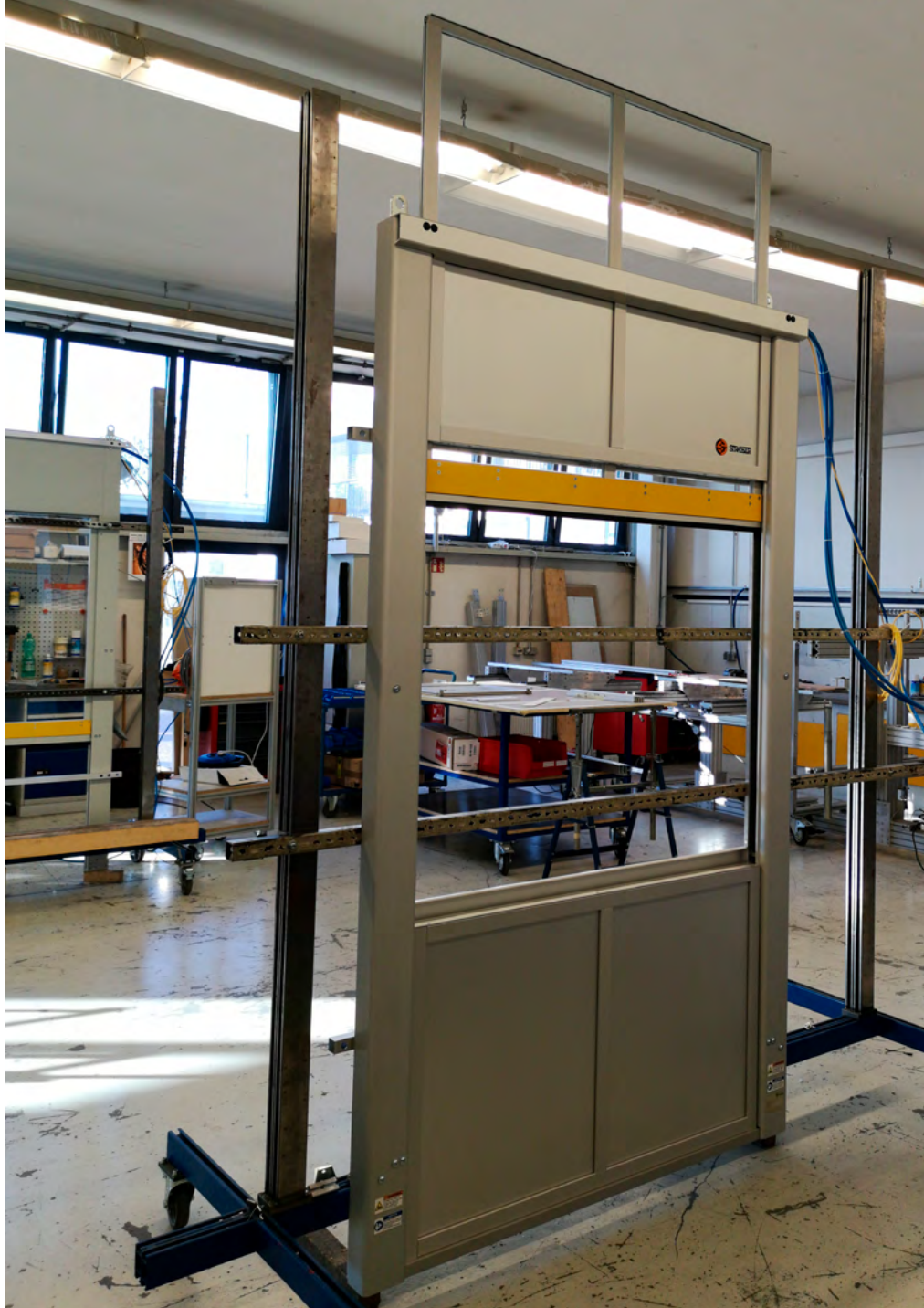
MecLock vertical safety window SFV.D-B01-P-1500-FMV – pneumatic actuator shortened upper panel – opened position – clear space above is still required (pane frame moves up)
