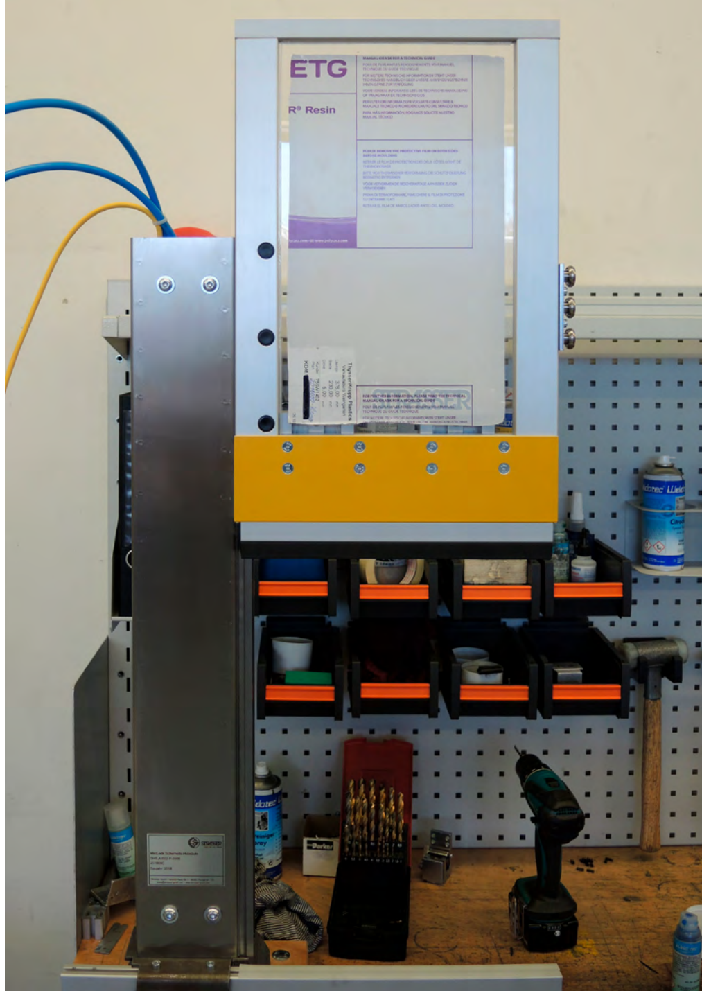
MecLock safety lifting column SHS.A – pneumatic actuator straight protective field – for small protection areas – table mounting opened position
