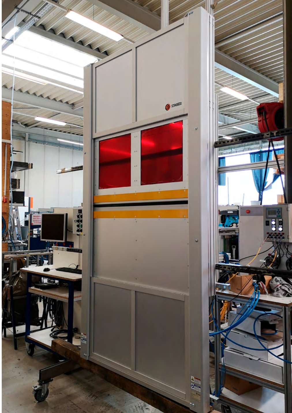
MecLock vertical safety window SFV.D-B01-P-1500-FM-...-FS21 – pneumatic actuator double-leaf design – light-protected with welding protection glasses for process monitoring
