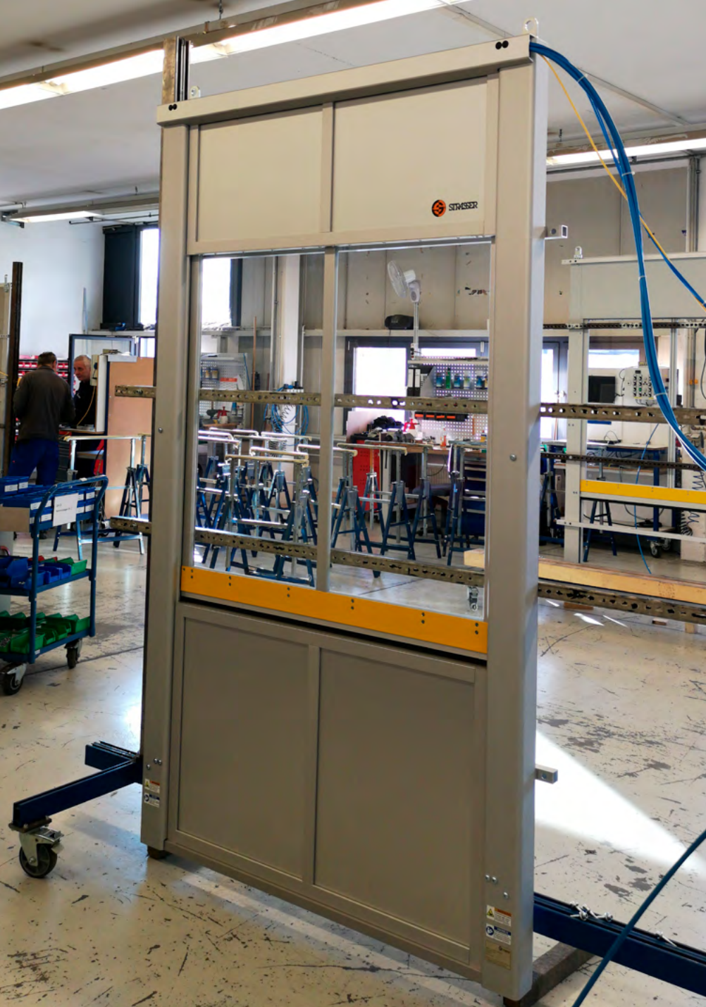
MecLock vertical safety window SFV.D-B01-P-1500-FMV – pneumatic actuator shortened upper panel – closed position
