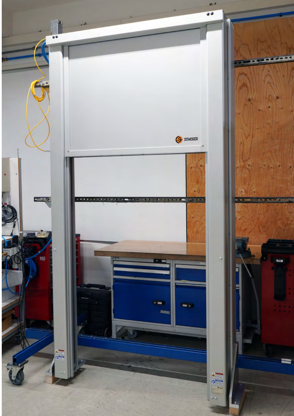
MecLock vertical safety window SFV.D-B01-P-1500 – pneumatic actuator with telescoping pane frame – closing direction from top to bottom completely retractable pane – barrier-free (without lower strut) – opened position
