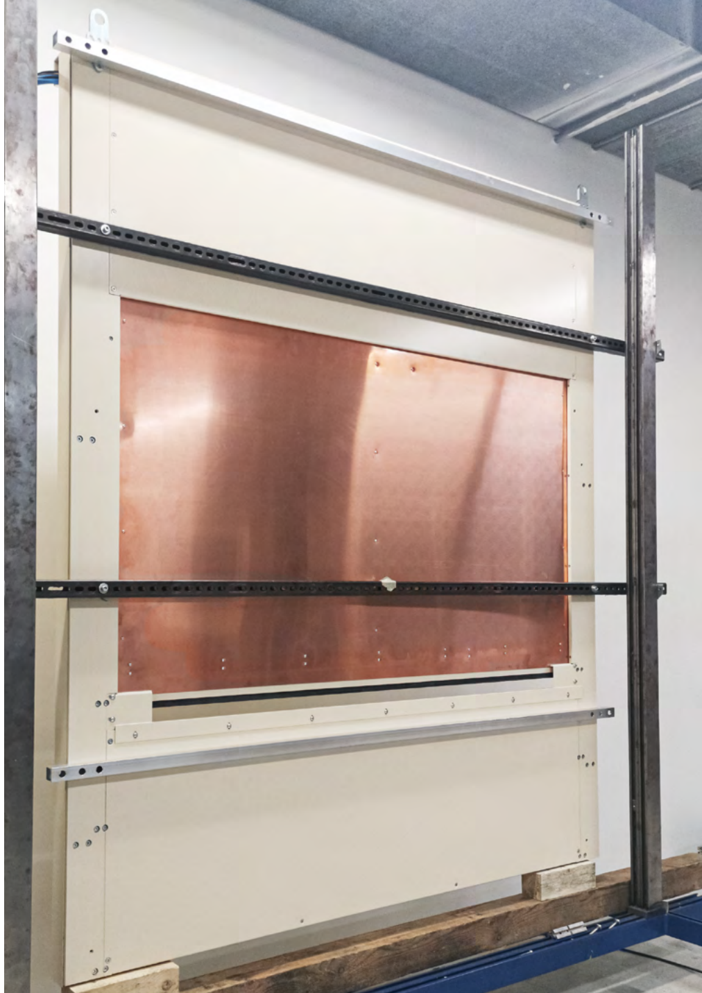
MecLock vertical safety window SFV.D-B01-P-1500-FMV – pneumatic actuator with shortened panel and lower strut – light-protected design rear view pane frame with copper sheet cover – closed position
