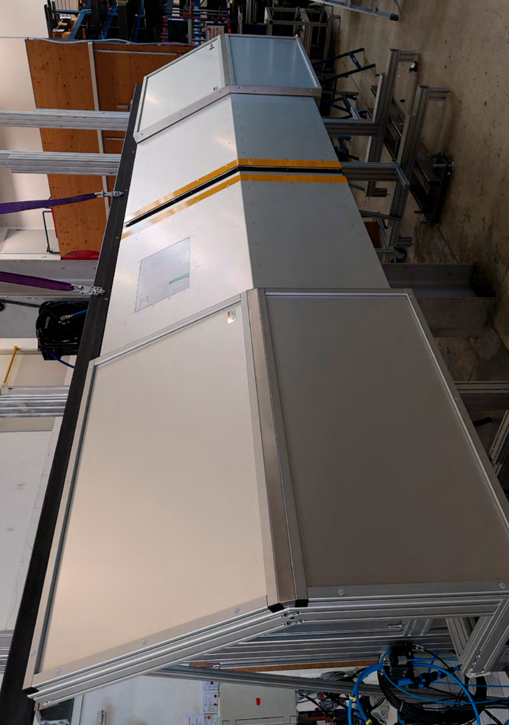
MecLock horizontal safety window SFH.E-B99-P-0750-FO-....FS21 pneumatic actuator – double-leaf version angled shape for friction welding machine – closed position
