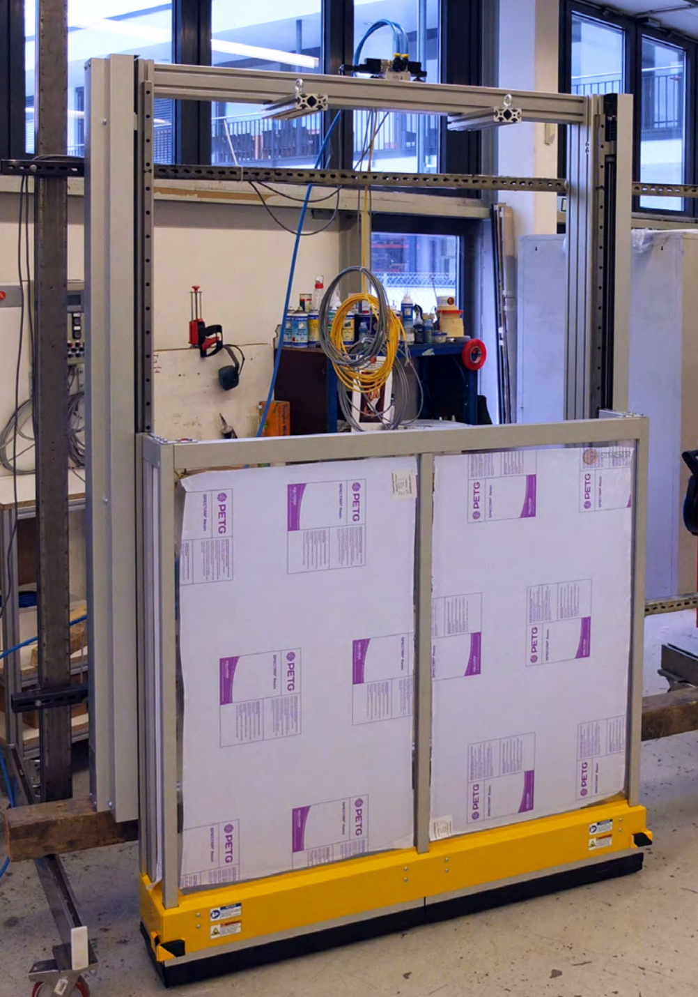
MecLock vertical safety window SFV.F-B30-P-2350-FO – pneumatic actuator protective field in U-shape – for medium and large protection areas – without upper panel protective field offset – clear space below is required (protective field moves down) closed position
