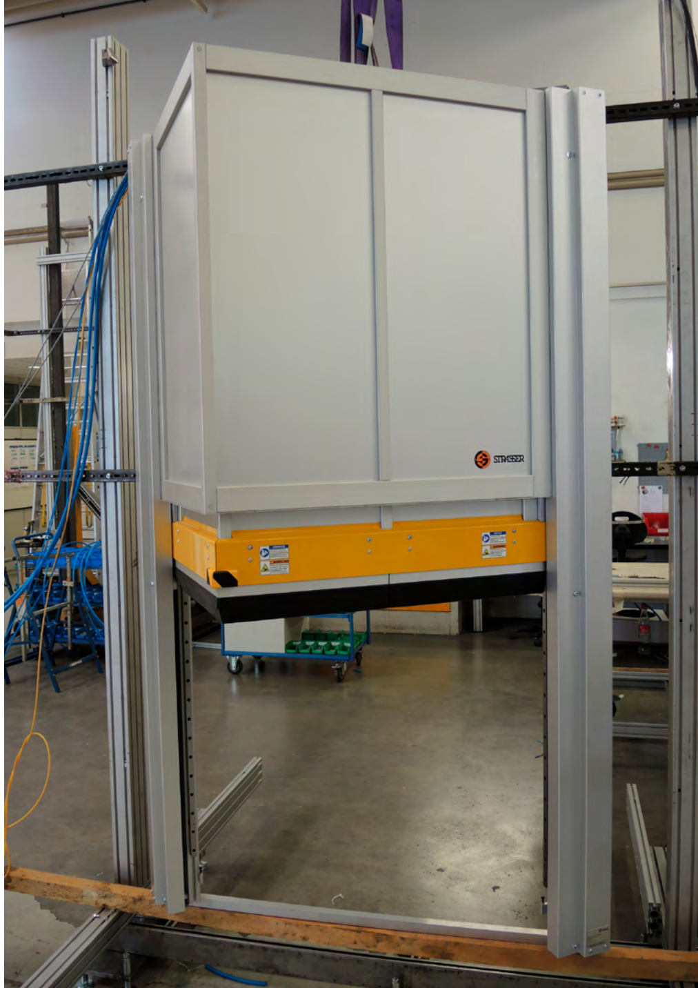
MecLock vertical safety window SFV.F-B10-P-2350-FO – pneumatic actuator protective field in L-shape – for medium and large protection areas – with upper panel opened position
