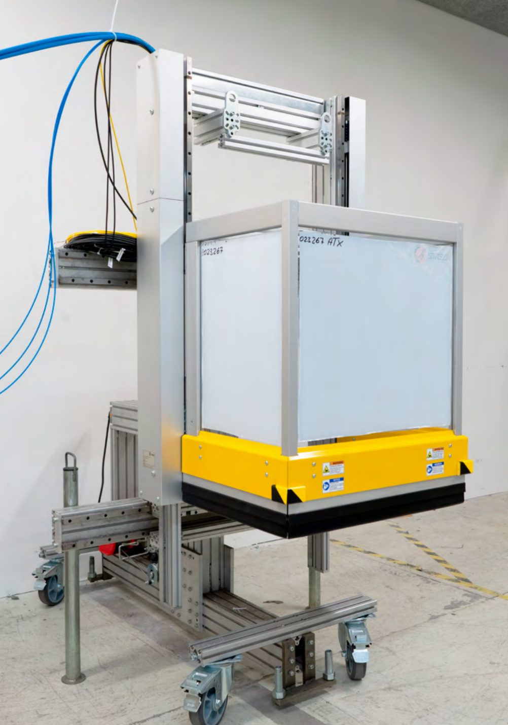
MecLock vertical safety window SFV.F-B30-P-2350-FO – pneumatic actuator protective field in U-shape – for medium and large protection areas without upper panel – closed position
