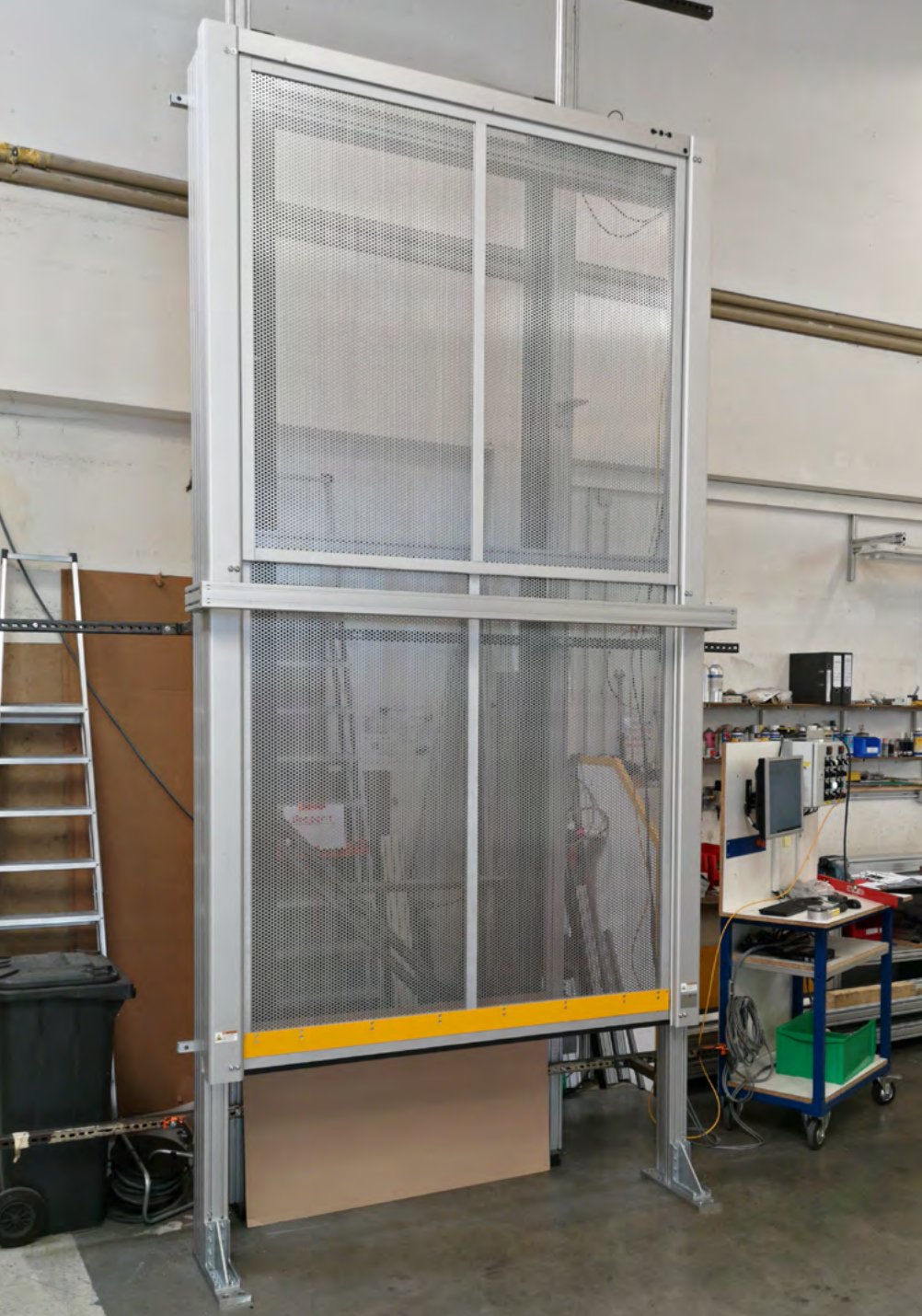
MecLock vertical safety window SFV.D-B01-E-4000 – servo-electric actuator floor standing model – pane and panel made of perforated metal sheets – base frame with impact protection to protect the pane frame from damage during loading and unloading
