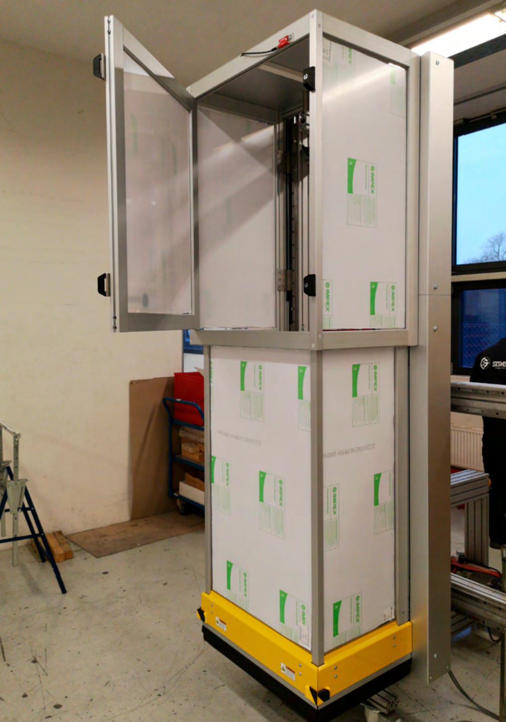
MecLock vertical safety window SFV.F-B30-E-7200-FO – servo-electric actuator protective field in U-shape for medium and large protection areas – panel with swing door opened penel door – closed position
