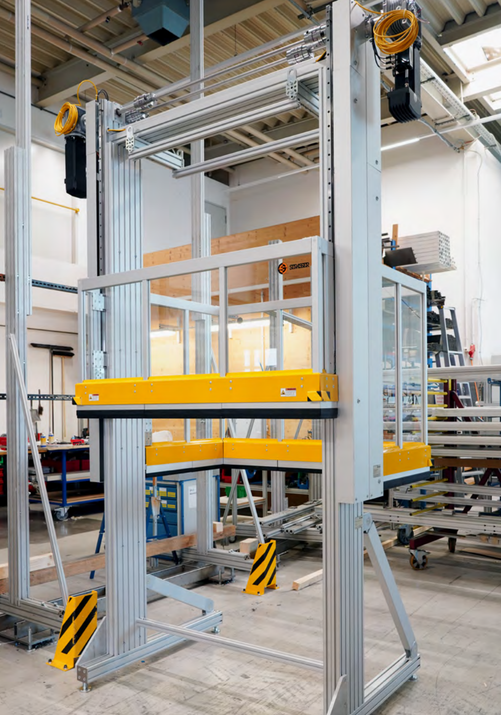
MecLock vertical safety window – servo-electric actuator Customized design with two separately controllable protective fields U-shaped protective fields for barrier-free accessibility from 3 sides closed position
