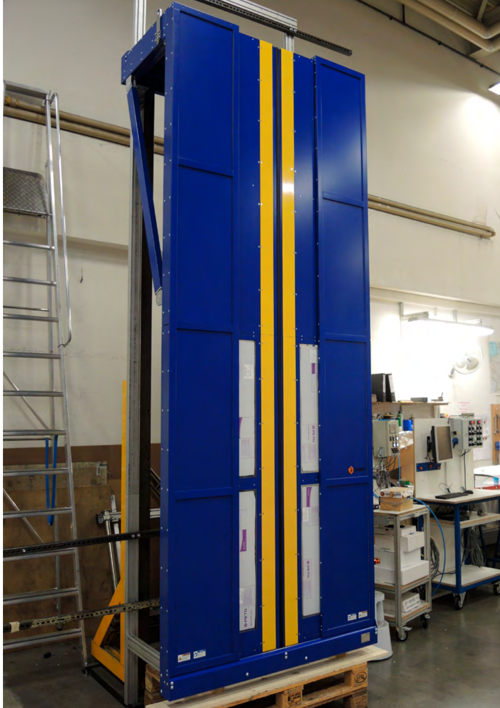
MecLock horizontal safety window SFH.E-B99-P-1500-FK-SA – pneumatic actuator double-leaf version in L-shape for hardening plant (induction hardening) splash water protected – closed position
