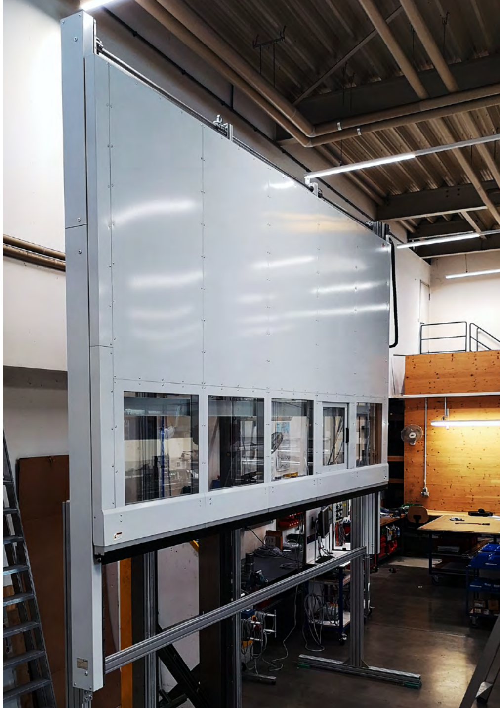
MecLock safeguard for dryers used to dry strands of thread – protection against mechanical hazards and for sealing off explosive substances – maximum machine side temperature 75 °C – opened position
