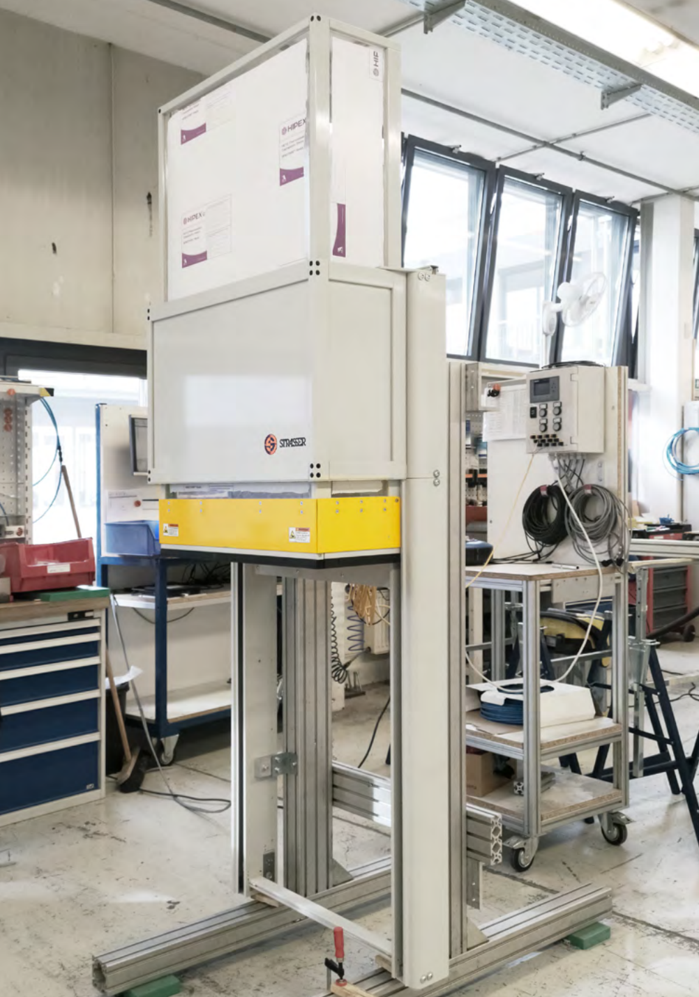
MecLock vertical safety window SFV.D-B30-E-4000-FOV – servo-electric actuator protective field in U-shape with shortened panel – for small and medium protection areas opened position
