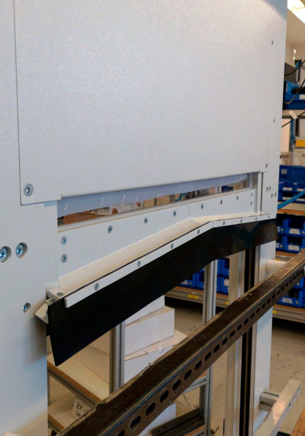
MecLock vertical safety window SFV.D-B01-P-1500-FM – pneumatic actuator splash water protected – drainage channel – opened position (rear view)
