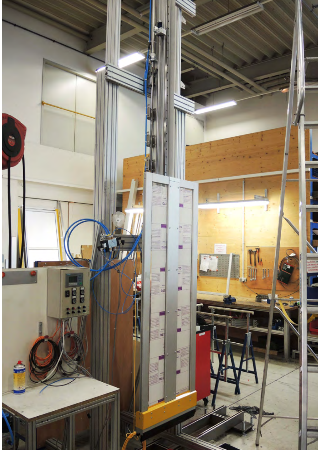
MecLock vertical safety window SFV.F-B99-P-1175-FO – pneumatic actuator straight protective field – clear space below is still required (protective field moves down freely) – closed position
