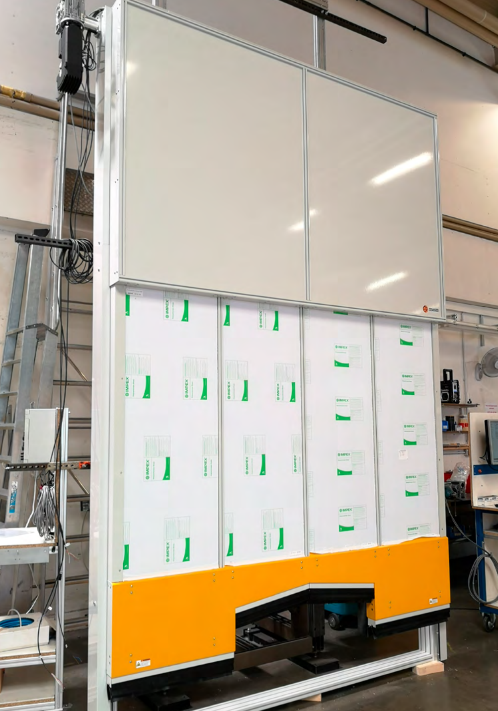
MecLock vertical safety window SFV.F-B01-E-7200-FO – servo-electric actuator dustproof design with contoured contact strip
