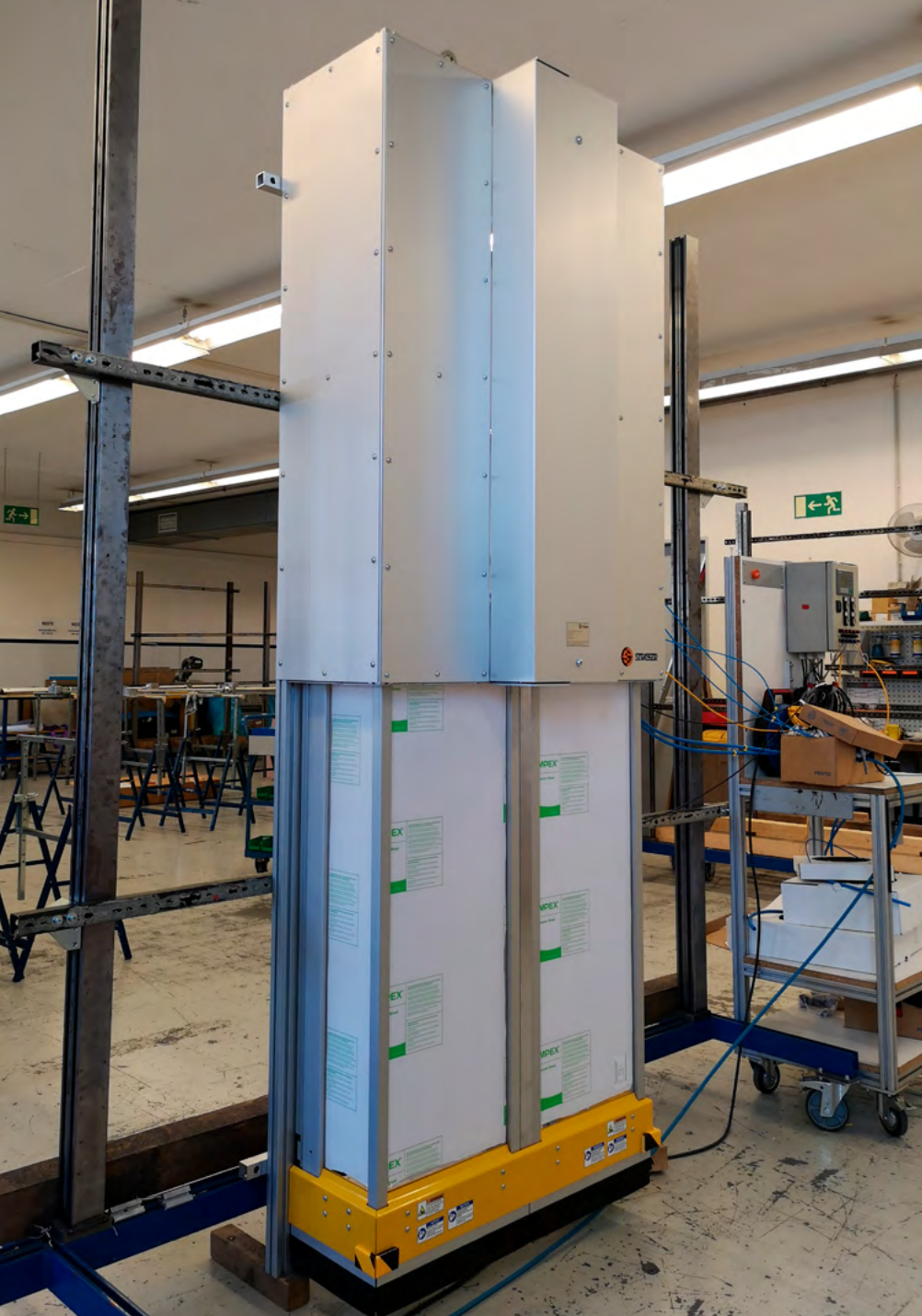
MecLock vertical safety window SFV.G-B30-P-1175-FO – pneumatic actuator protective field in U-shape – center drive for minimal overall width access for maintenance from the front – closed position
