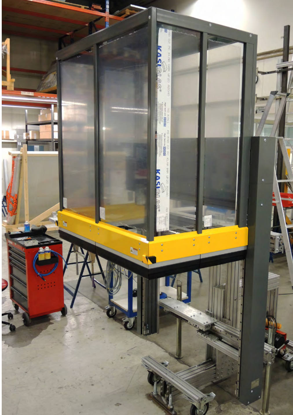
MecLock vertical safety window SFV.F-B30-E-7200-FO – servo-electric actuator protective field in U-shape for medium and large protection areas – antistatic version with protective field cover on top – shortened design clear space above is still required (protective field moves up) – opened position
