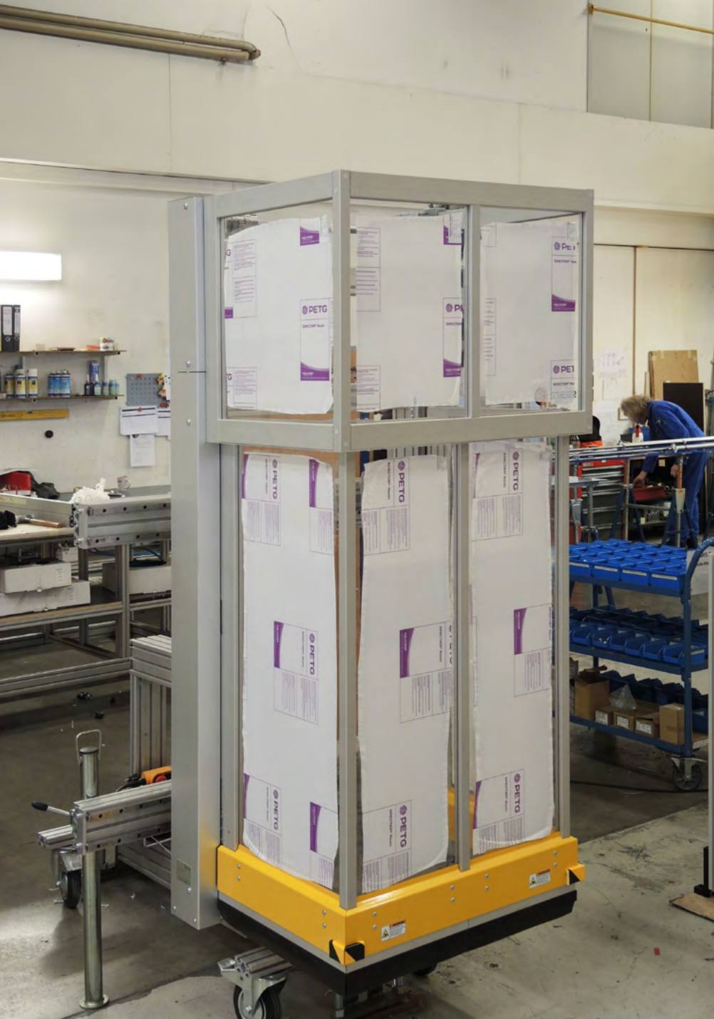
MecLock vertical safety window SFV.F-B30-P-2350-FO – pneumatic actuator protective field in U-shape – for medium and large protection areas – with shortened upper panel – clear space above is still required (protective field moves up) – closed position
