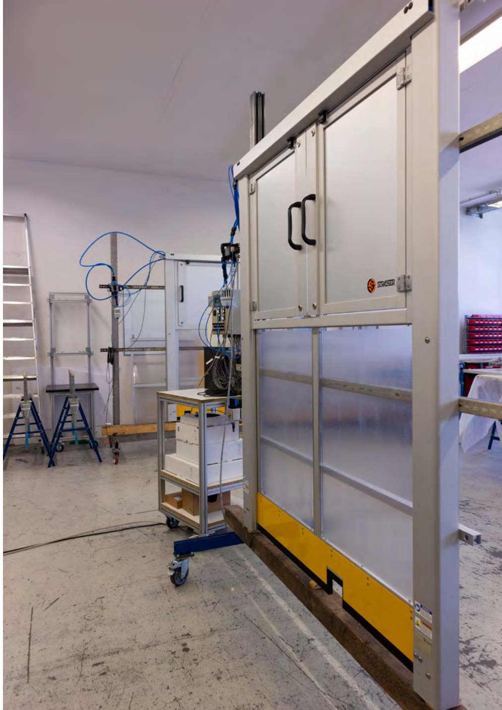
MecLock vertical safety window SFV.D-B01-P-1500-FO – pneumatic actuator with contoured contact strip – monitored panel doors for maintenance of the machine behind
