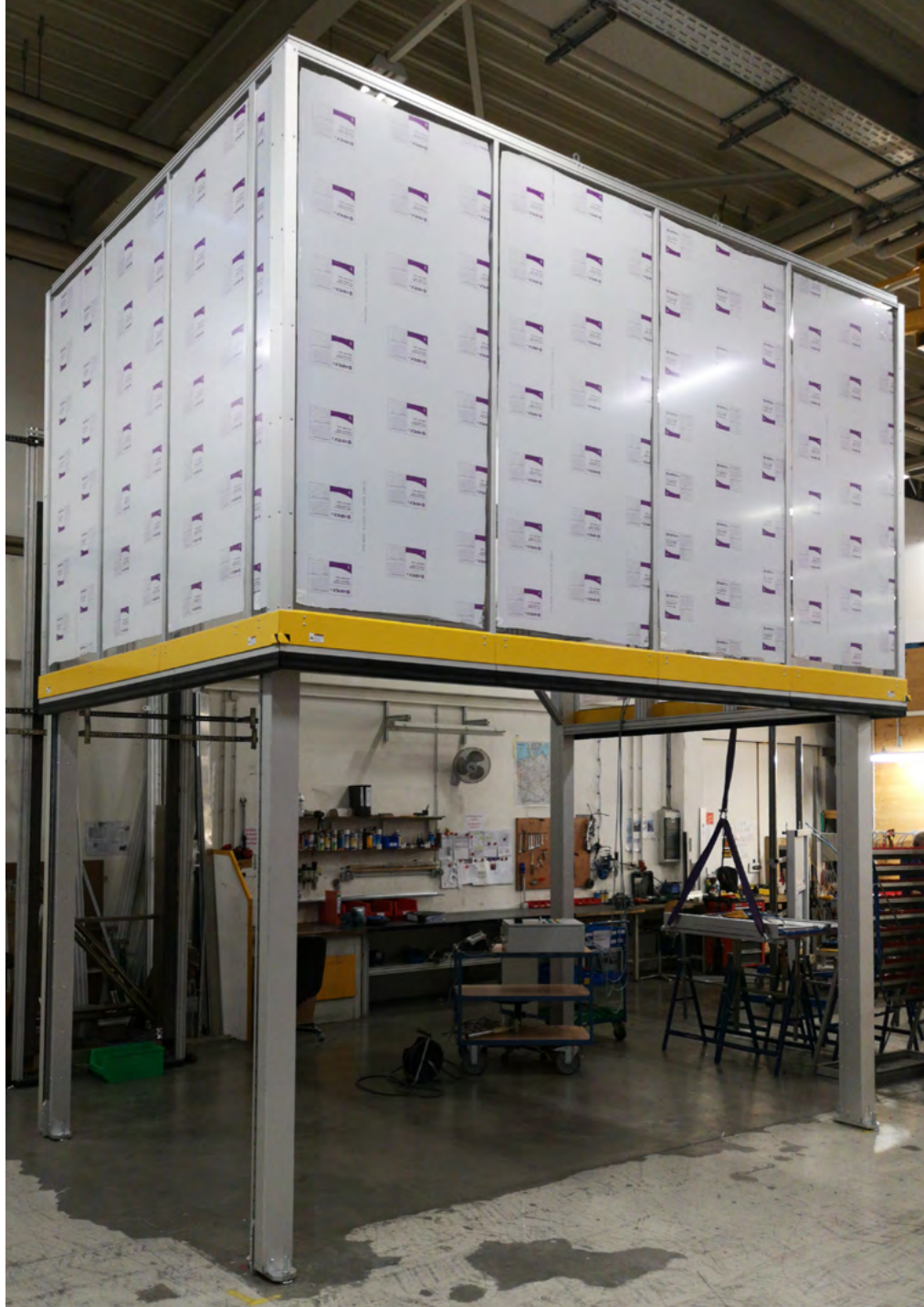
MecLock vertical safety window SFV.F-B99-E-14400-FO – servo-electric actuator protective field in U-shape for barrier-free access from 3 sides customized design for test bench in medical industry opened position
