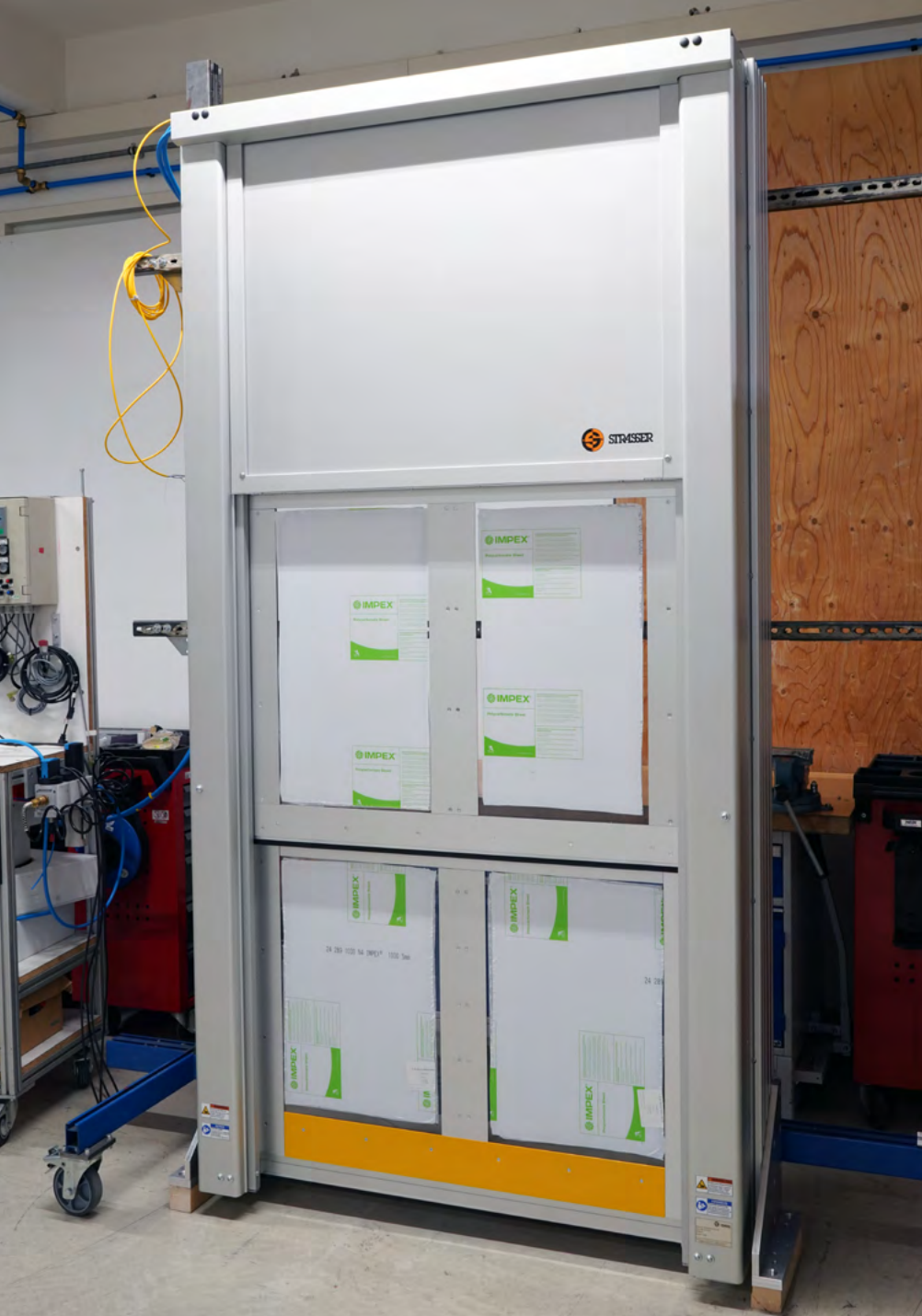
MecLock vertical safety window SFV.D-B01-P-1500 – pneumatic actuator with telescoping pane frame – closing direction from top to bottom completely retractable pane – barrier-free (without lower strut) – closed position
