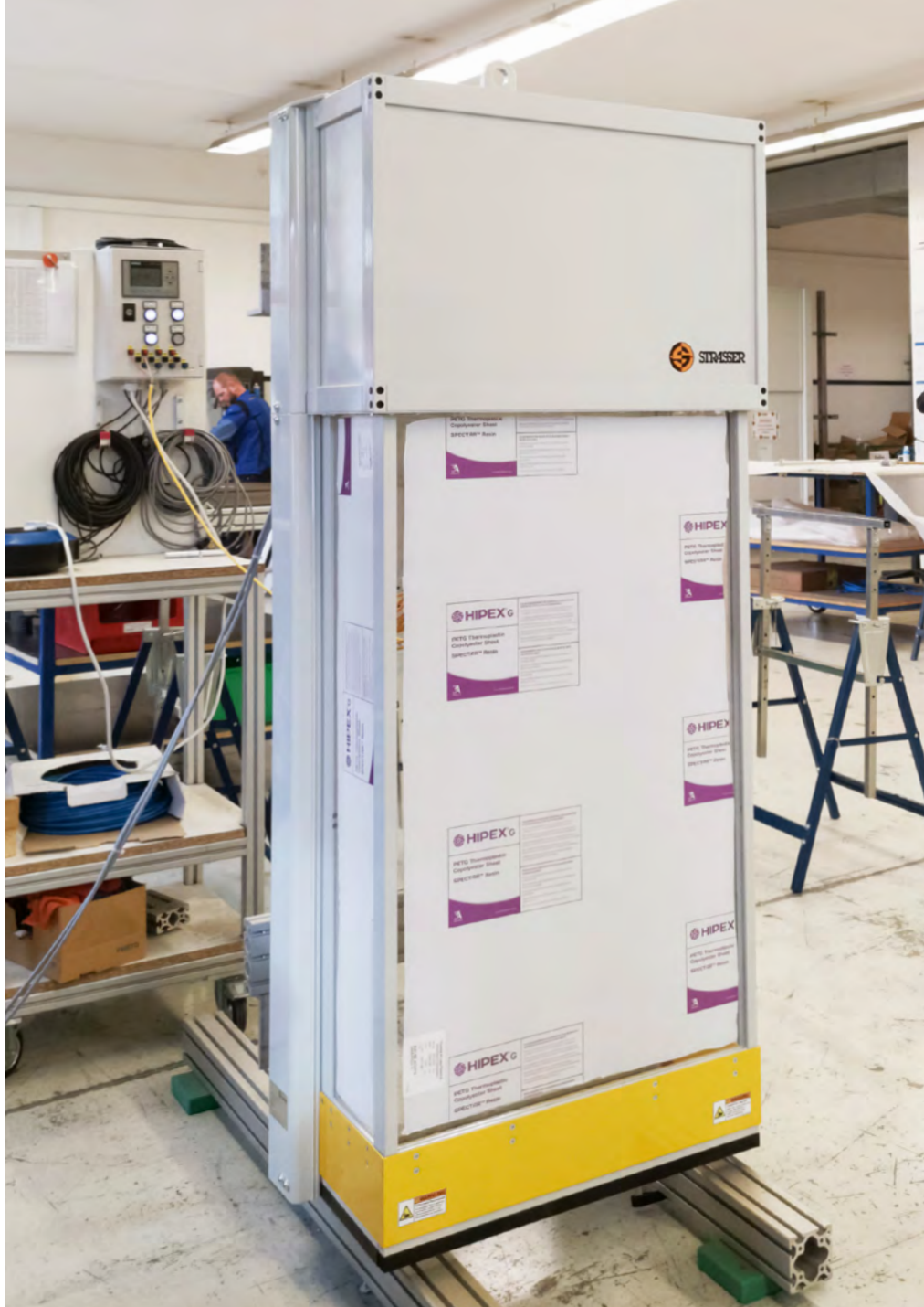
MecLock vertical safety window SFV.D-B30-E-4000-FOV – servo-electric actuator protective field in U-shape with shortened panel – for small and medium protection areas closed position
