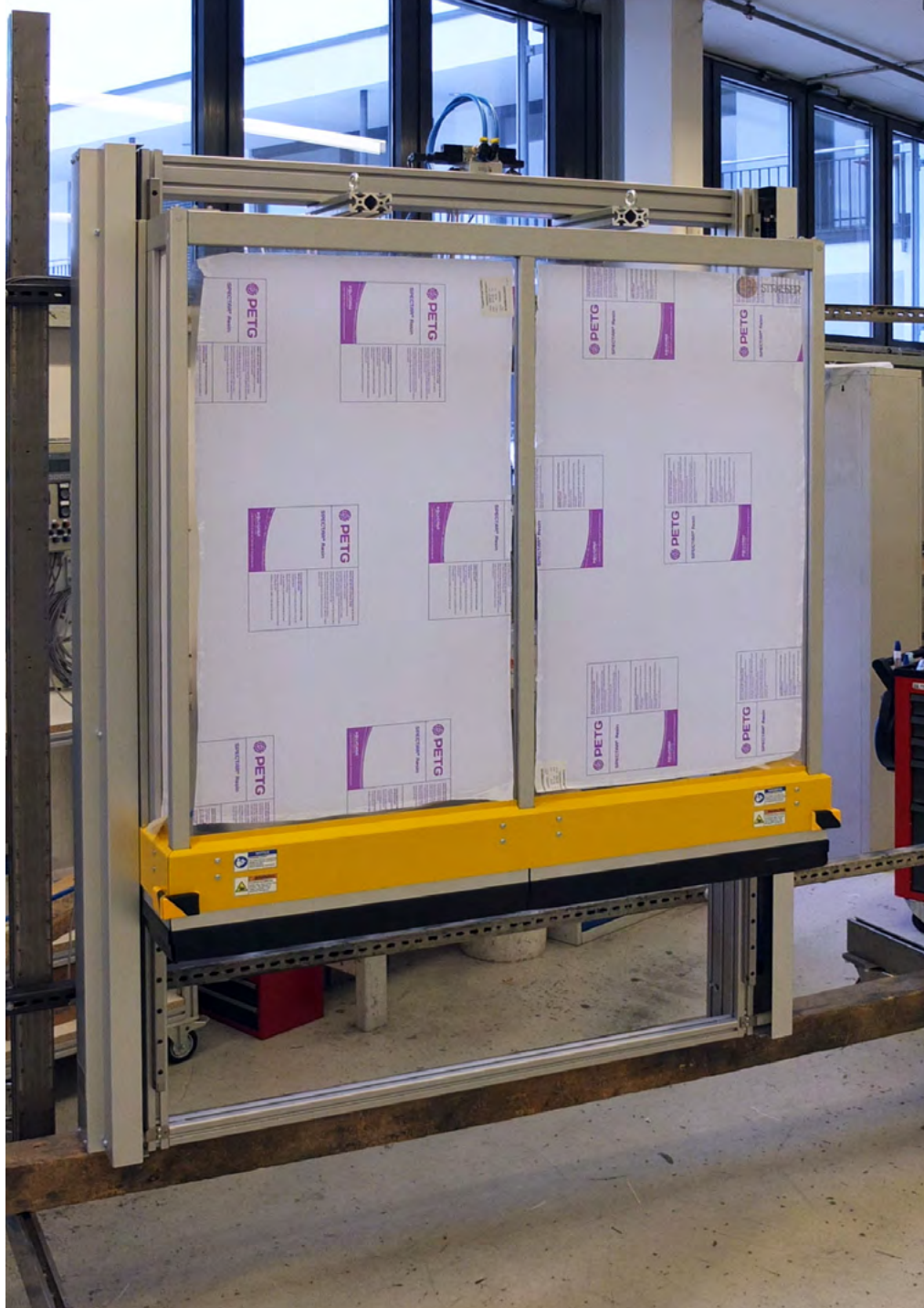
MecLock vertical safety window SFV.F-B30-P-2350-FO – pneumatic actuator protective field in U-shape – for medium and large protection areas – without upper panel protective field offset – clear space below is required (protective field moves down) opened position
