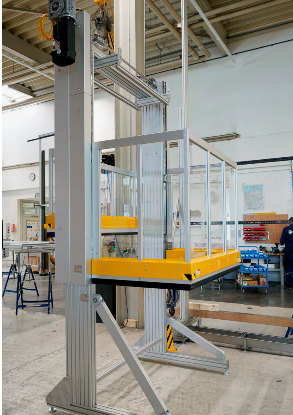
MecLock vertical safety window – servo-electric actuator Customized design with two separately controllable protective fields U-shaped protective fields for barrier-free accessibility from 3 sides opened position
