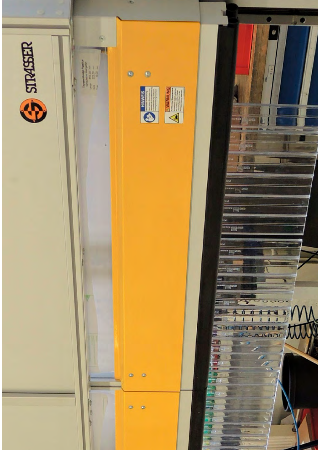
MecLock vertical safety window SFV.F-B99-P-2350-FM – pneumatic actuator separately controllable curtain with individually mounted slats for isolation of oversized workpieces protruding from the machine
