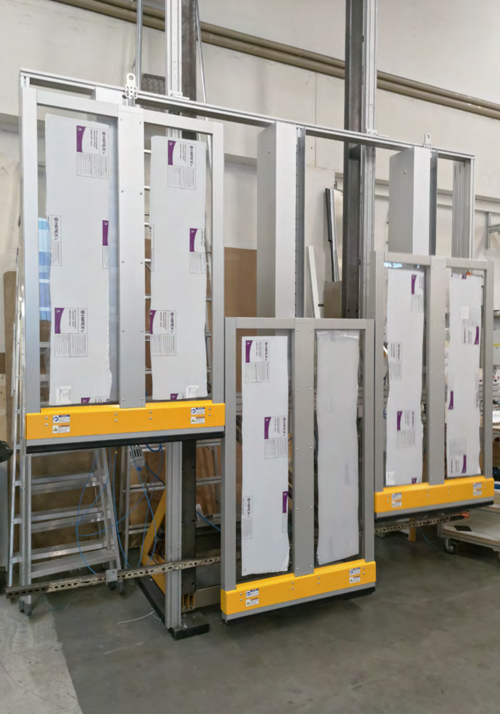
MecLock vertical safety window SFV.G-B99-P – pneumatic actuator 3 individually controllable safety windows on a common base frame protective field moves down freely
