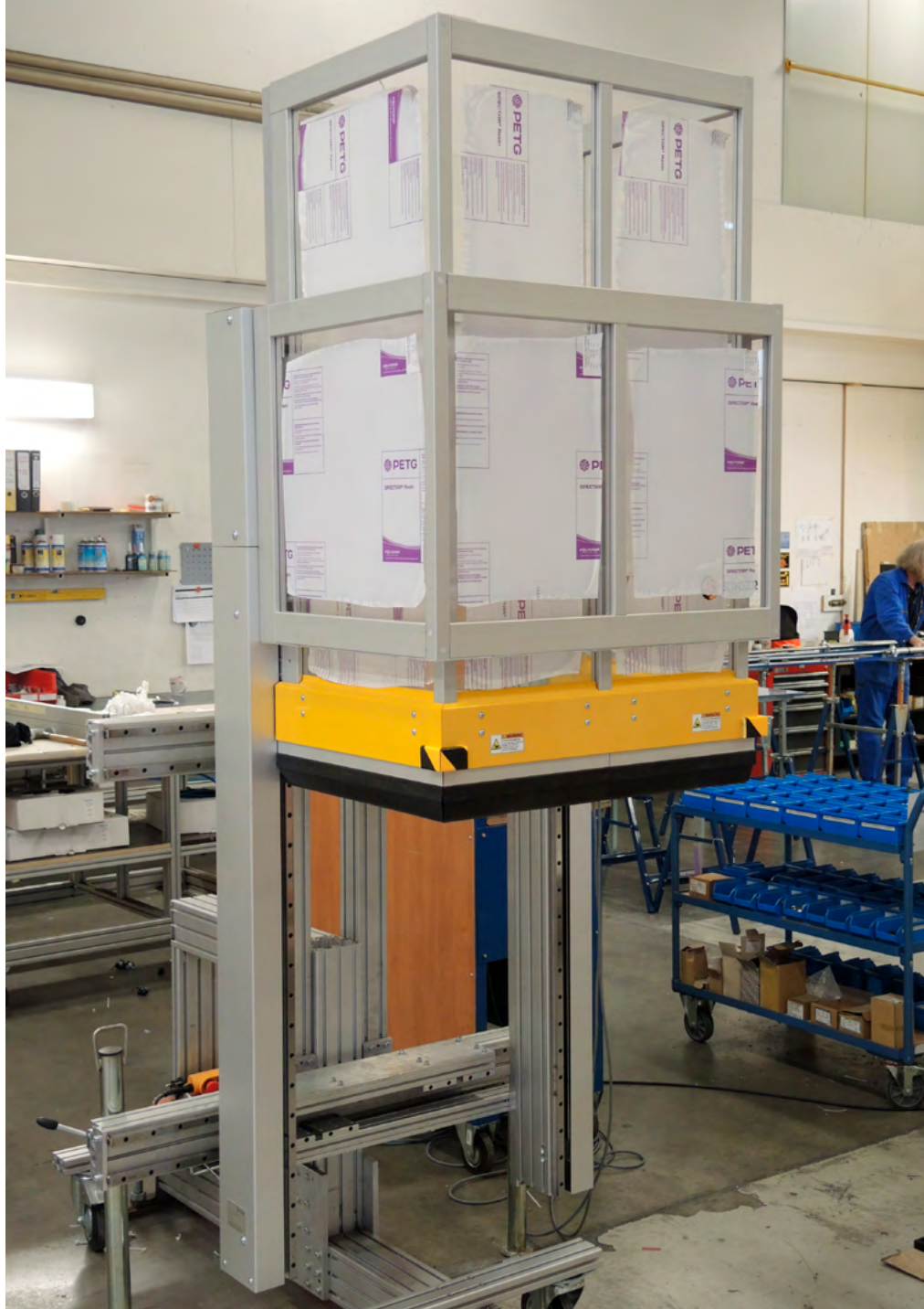
MecLock vertical safety window SFV.F-B30-P-2350-FO – pneumatic actuator protective field in U-shape – for medium and large protection areas – with shortened upper panel – clear space above is still required (protective field moves up) – opened position
