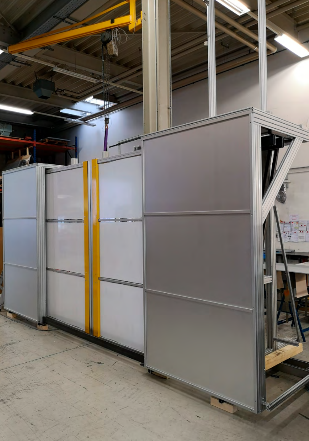
MecLock horizontal safety window SFH.E-B99-E-3600-...-FS21 servo-electric actuator – double-leaf version – L-shape for large protection areas closed position
