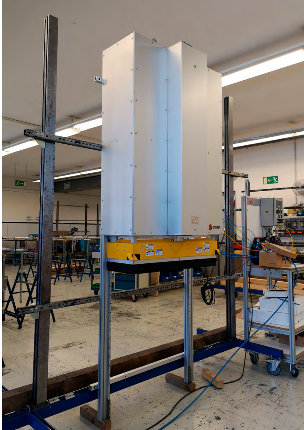
MecLock vertical safety window SFV.G-B30-P-1175-FO – pneumatic actuator protective field in U-shape – center drive for minimal overall width – aluminium panel access for maintenance from the front – opened position
