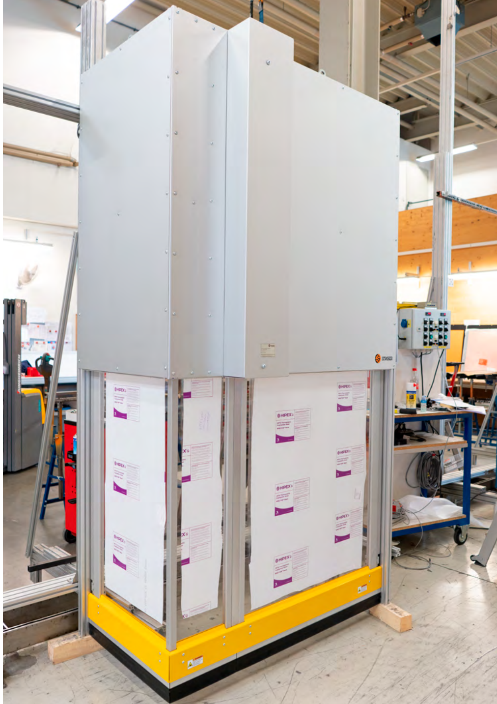
MecLock vertical safety window SFV.G-B10-E-3600-FO – servo-electric actuator protective field in L-shape – center drive for minimal overall width access for maintenance from the front – closed position
