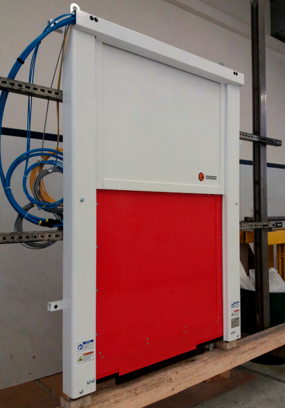
MecLock vertical safety window SFV.D-B01-P-1500-FO – pneumatic actuator soundproof design with contoured contact strip for adaption of the closing edge to the machine contour
