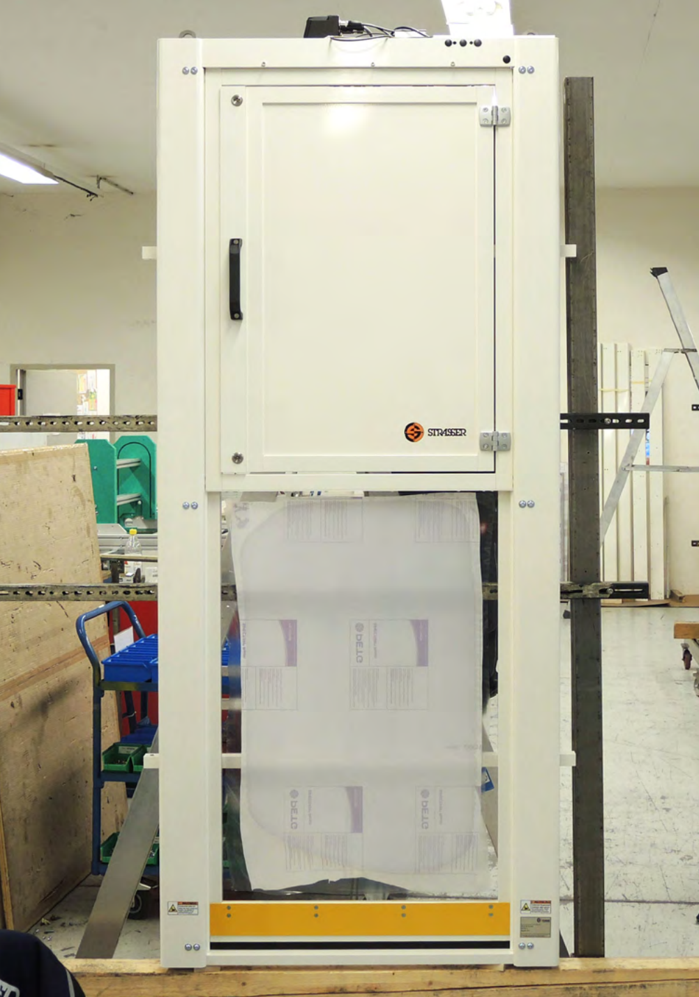
MecLock vertical safety window SFV.D-B01-E-4000-FM – servo-electric actuator with panel door for access and maintenance of the machine behind
