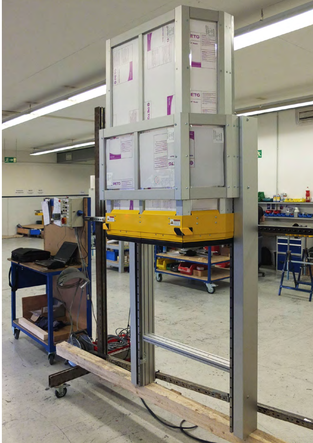
MecLock vertical safety window SFV.F-B99-E-7200-FO – servo-electric actuator protective field in U-shape – for medium and large protection areas customized protective field (adapted to the machine contour) – shortened design clear space above is still required (protective field moves up) – opened position
