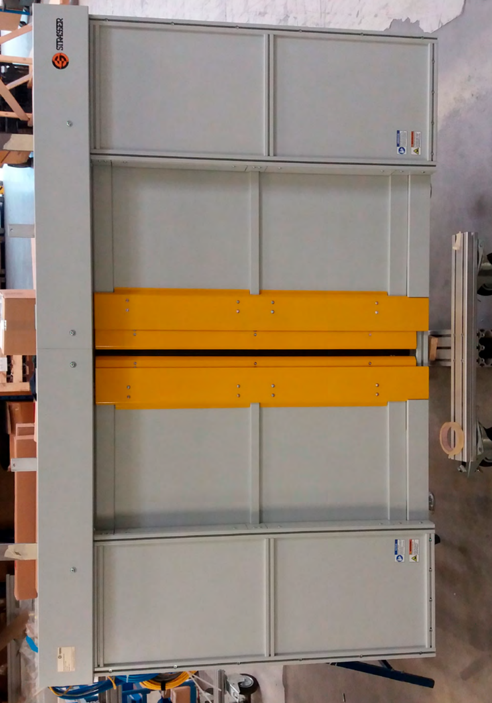
MecLock horizontal safety window SFH.E-B01-P-0750-FO-....-FS21 pneumatic actuator – double-leaf version – light-protected design
