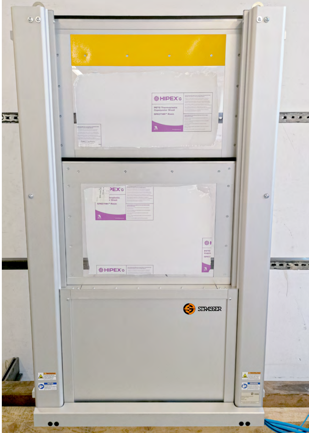
MecLock vertical safety window SFV.D-B01-P-1500-FO – pneumatic actuator with telescoping pane frame – closing direction from bottom to top completely retractable pane – barrier-free on the top – closed position
