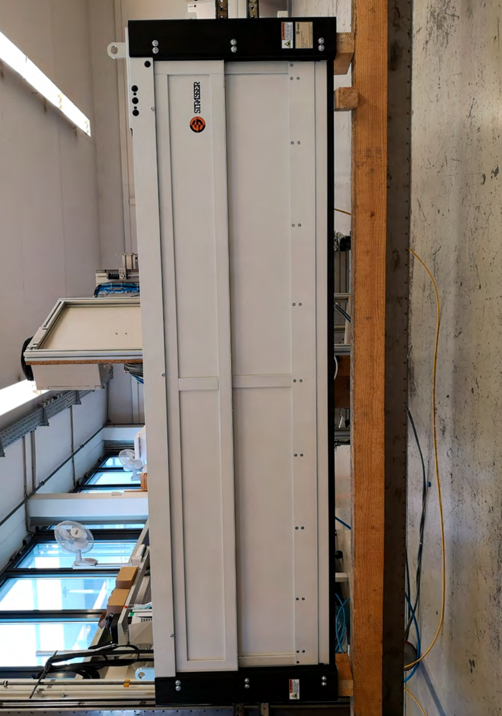
MecLock vertical safety window SFV.D-B01-E-4000-FO – servo-electric actuator light-protected design – small stroke and large clear width
