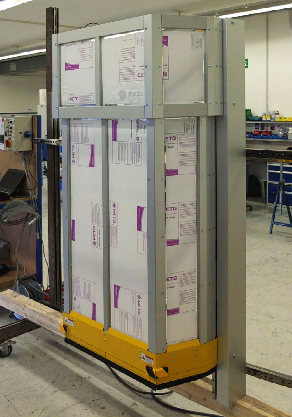
MecLock vertical safety window SFV.F-B99-E-7200-FO – servo-electric actuator protective field in U-shape – for medium and large protection areas customized protective field (adapted to the machine contour) – shortened design clear space above is still required (protective field moves up) – closed position
