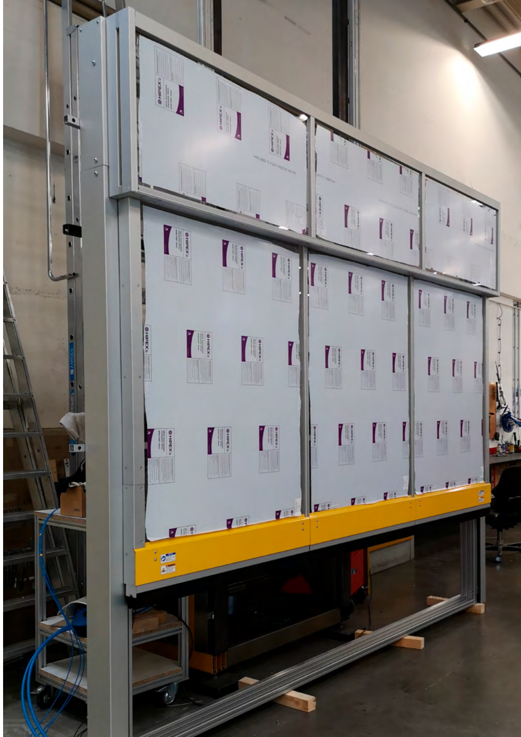
MecLock vertical safety window SFV.F-B01-P-2350-FM – pneumatic actuator for large protection areas – shortened panel
