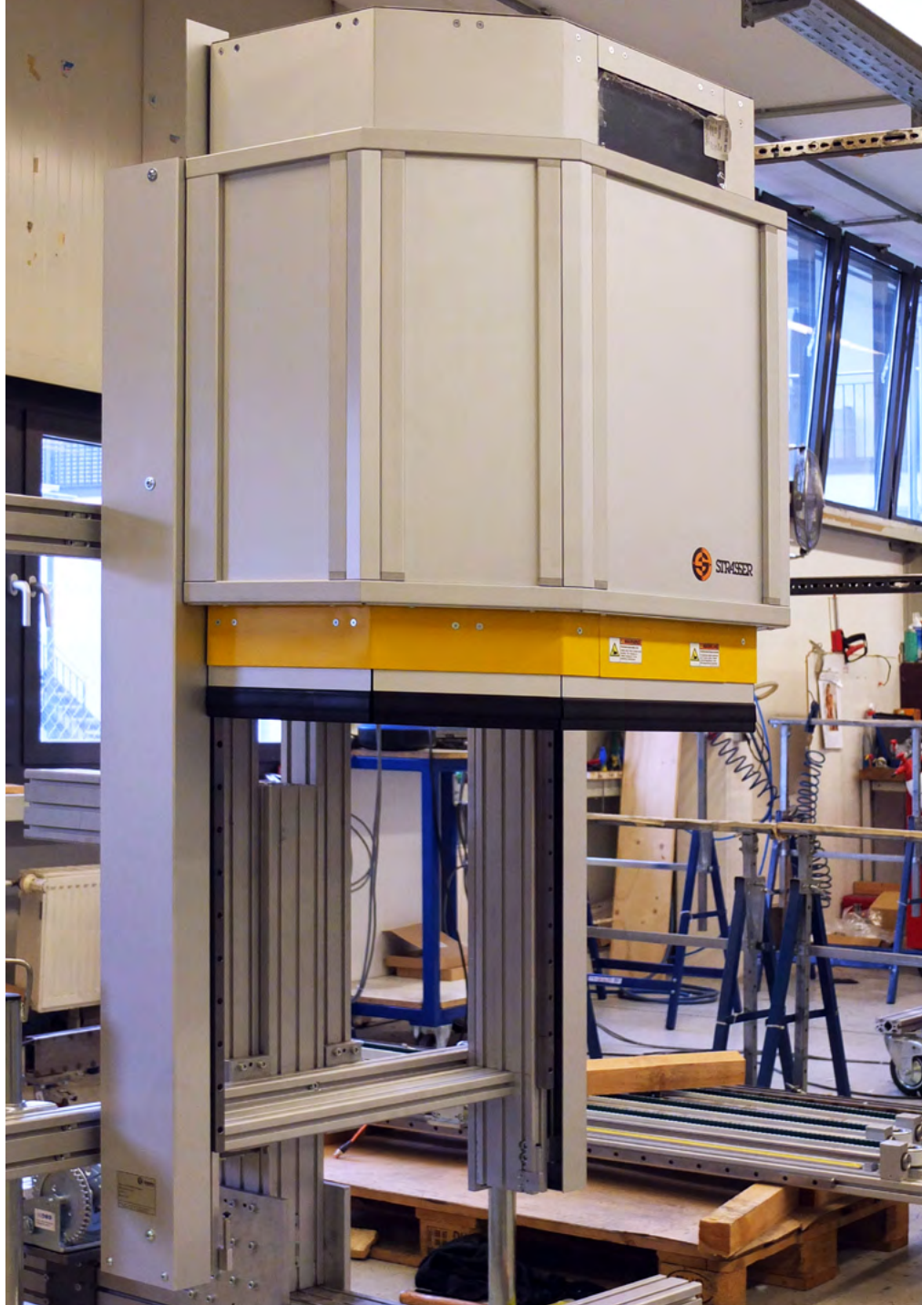
MecLock vertical safety window SFV.F-B99-E-7200-FO – servo-electric actuator center drive – customized protective field for engine injection test station sound insulated and optimized for use in potentially explosive environments (no complete explosion protection) – opened position
