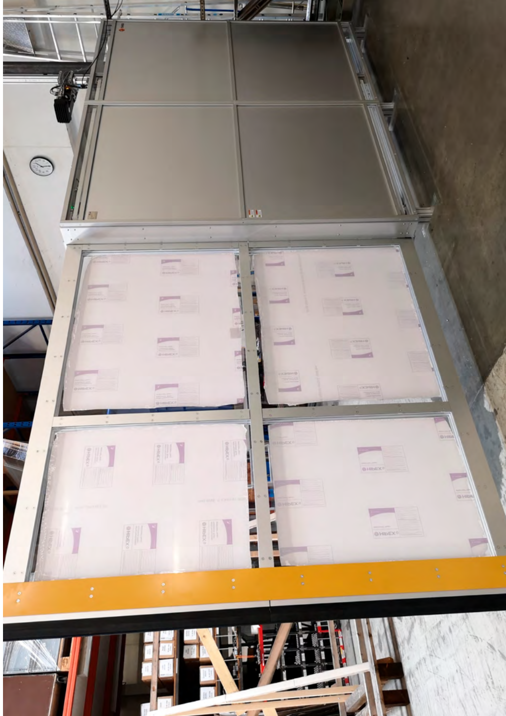
MecLock horizontal safety window SFH.E-B99-E – servo-electric actuator self-supporting single-leaf version on posts – barrier-free for loading with crane or forklift truck (door leaf moves out freely) – closed position
