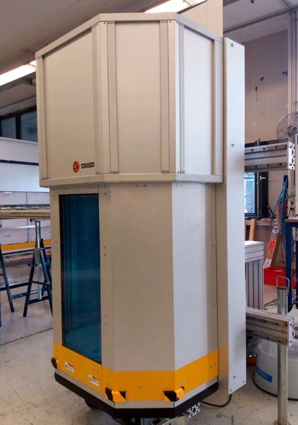
MecLock vertical safety window SFV.F-B99-E-7200-FO – servo-electric actuator center drive – customized protective field for engine injection test station sound insulated and optimized for use in potentially explosive environments (no complete explosion protection) – closed position
