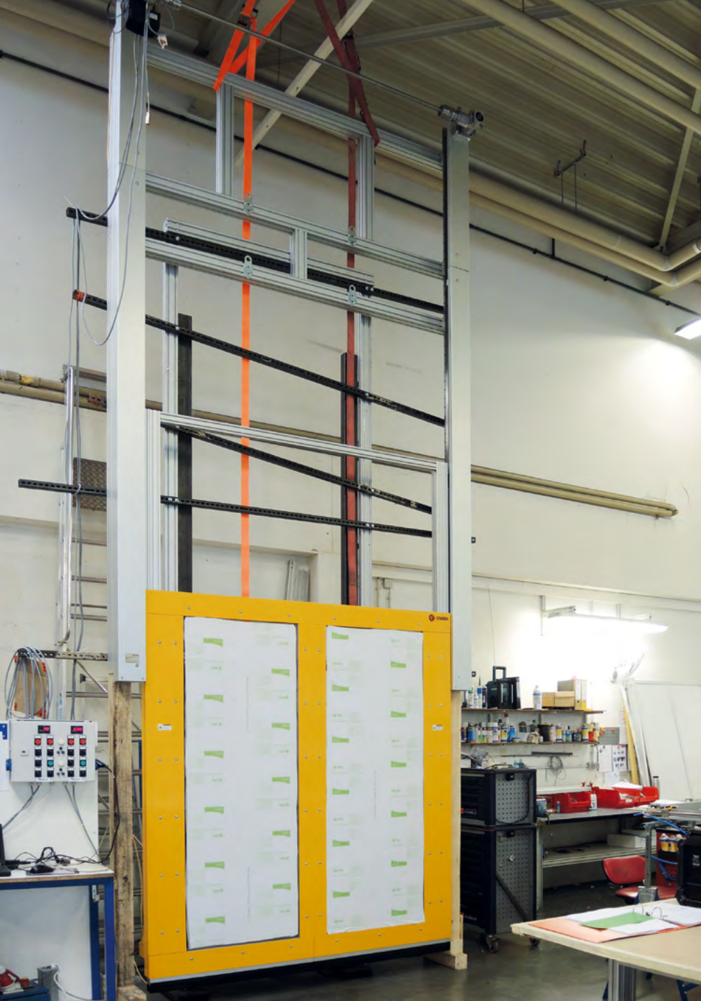
MecLock vertical safety window SFV.F-B99-E-7200-FO – servo-electric actuator large press retrofit project – service life extension and adaptation to current safety standards clear space below is still required (pane frame moves down freely)
