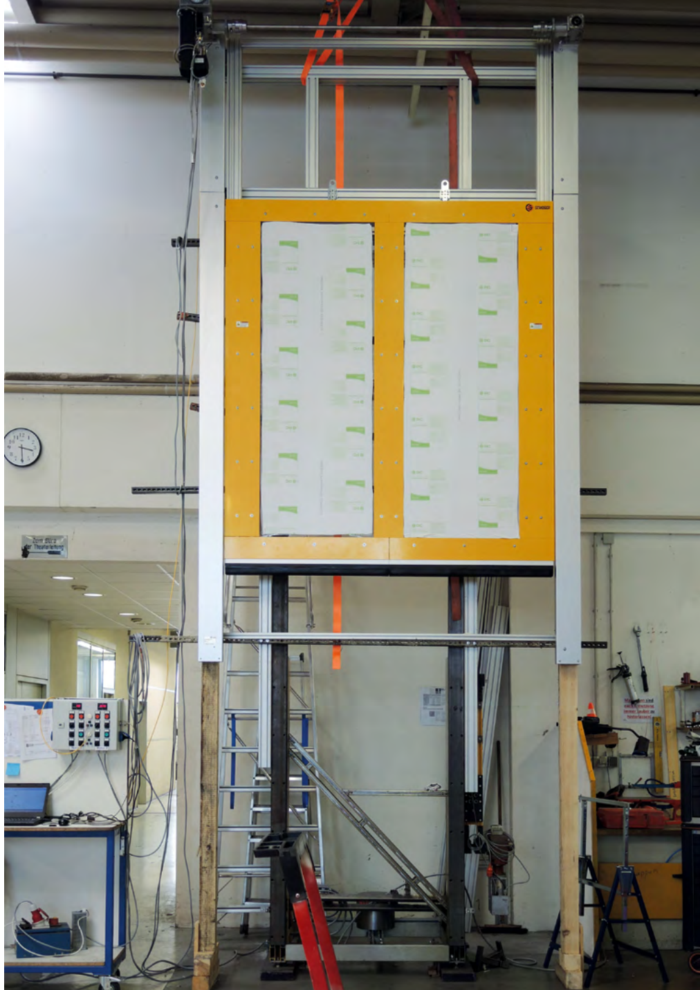
MecLock vertical safety window SFV.F-B99-E-7200-FO – servo-electric actuator large press retrofit project – opened position
