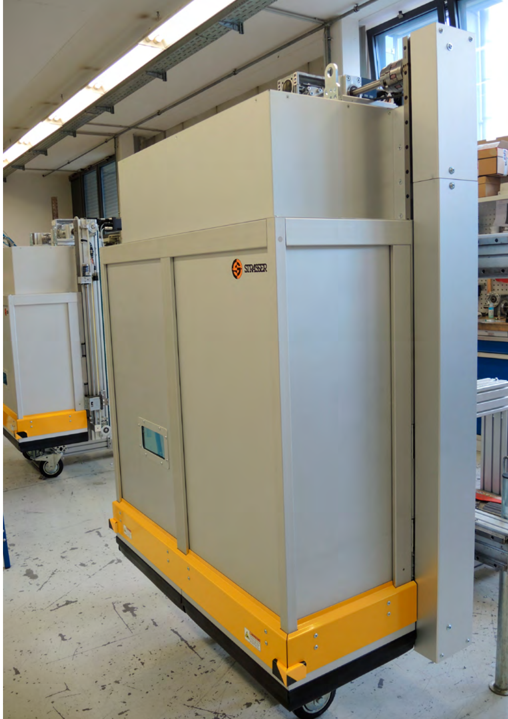
MecLock vertical safety window SFV.F-B99-E-7200-FO – servo-electric actuator center drive – protective field in U-shape for medium and large protection areas light-protected in labyrinth design – process window with laser protection glass shortened design – clear space above is still required (protective field moves up)
