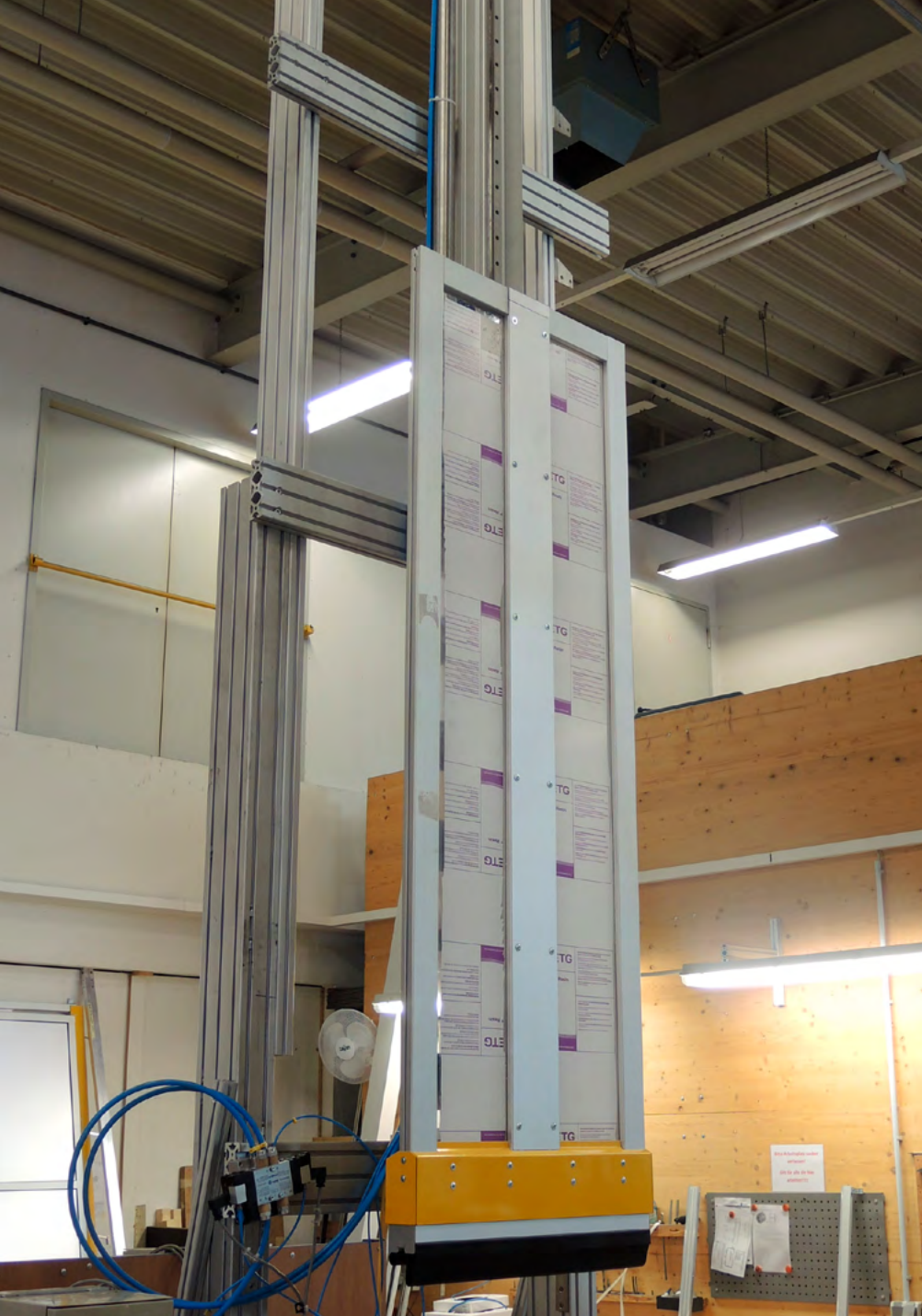
MecLock vertical safety window SFV.F-B99-P-1175-FO – pneumatic actuator straight protective field – clear space below is still required (protective field moves down freely) – opened position
