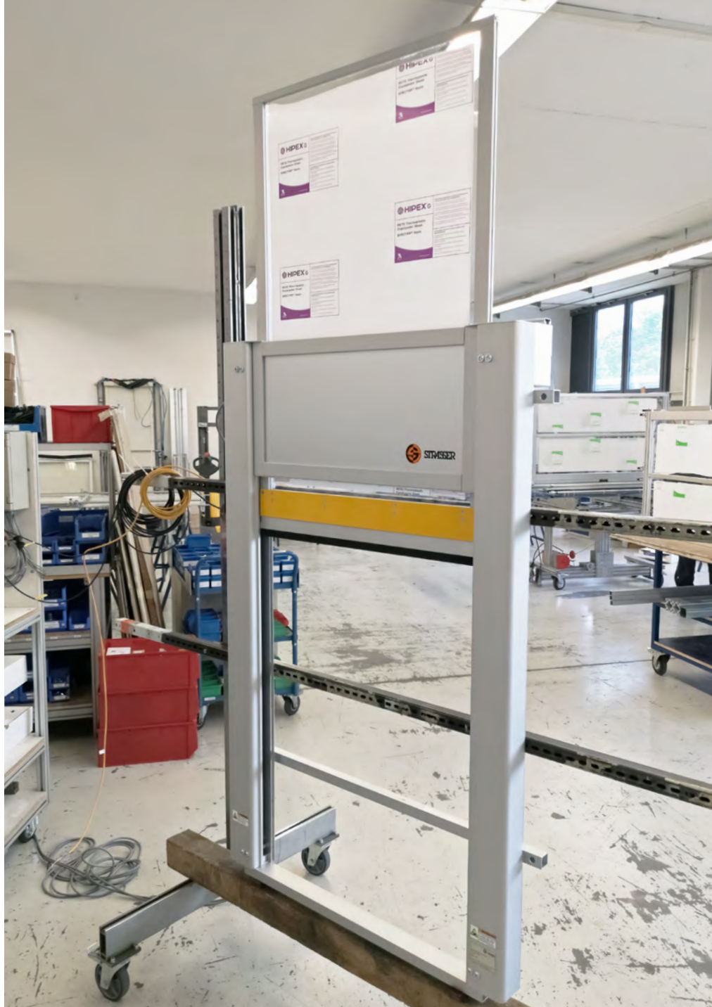
MecLock vertical safety window SFV.D-B01-E-4000-FOV – servo-electric actuator without lower strut – shortened upper panel – opened position
