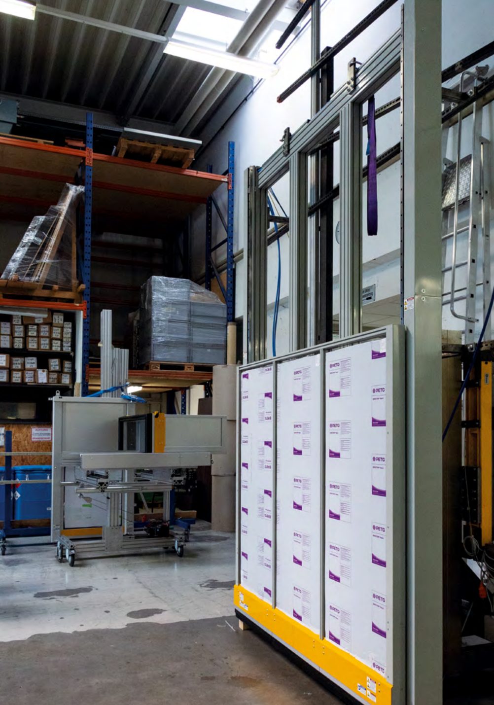
MecLock vertical safety window SFV.F-B01-P-2350-FM – pneumatic actuator for large protection areas – without upper panel
