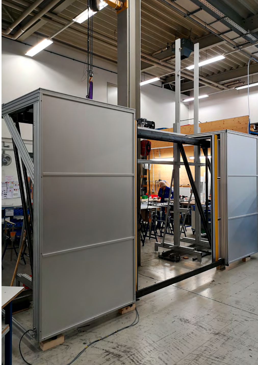
MecLock horizontal safety window SFH.E-B99-E-3600-...-FS21 servo-electric actuator – double-leaf version – L-shape for large protection areas opened position
