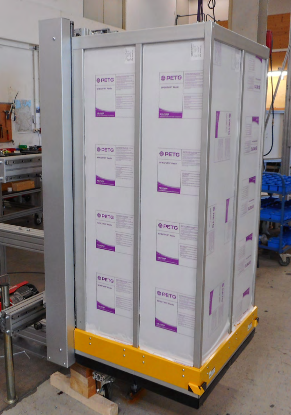
MecLock vertical safety window SFV.F-B30-E-7200-FO – servo-electric actuator protective field in U-shape – for medium and large protection areas – center drive continuous protective field without upper panel – shortened design clear space above is still required (protective field moves up)
