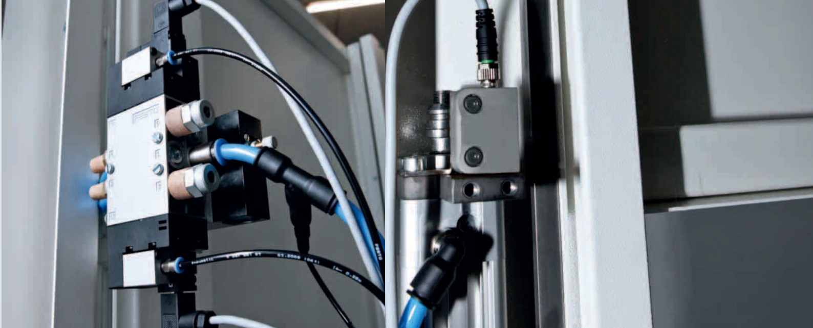
Powerful pneumatic cylinders DNCB from Festo move specially designed safety doors at high speeds of up to two metres a second.
