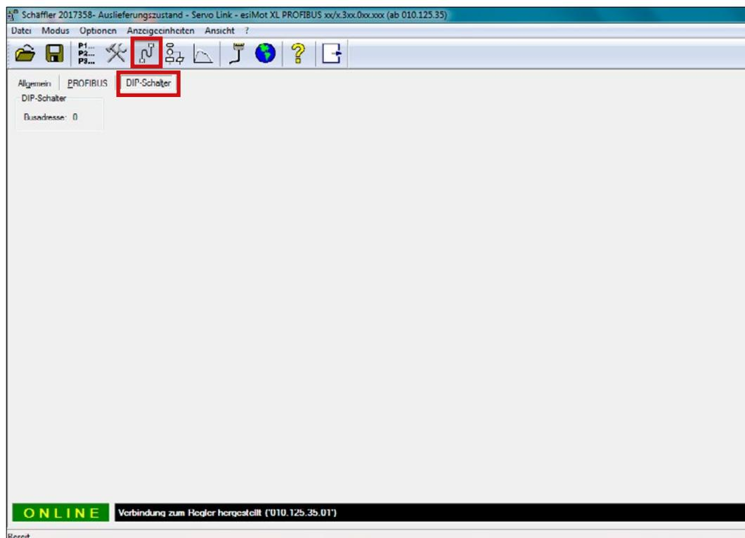
Fig. 27: 'DIP-Switch'-tab in 'Diagnostics'-screen (only with PROFIBUS DP interface)
