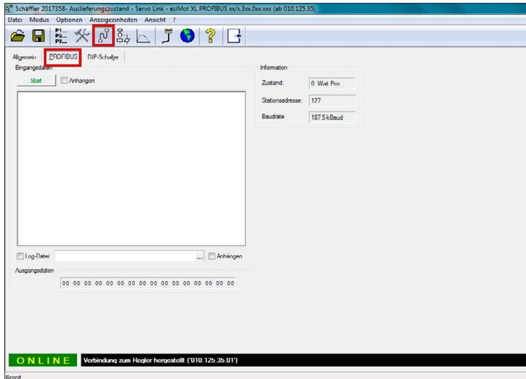
Fig. 26: 'PROFIBUS'-tab in 'Diagnostics'-screen (only with PROFIBUS DP interface)
