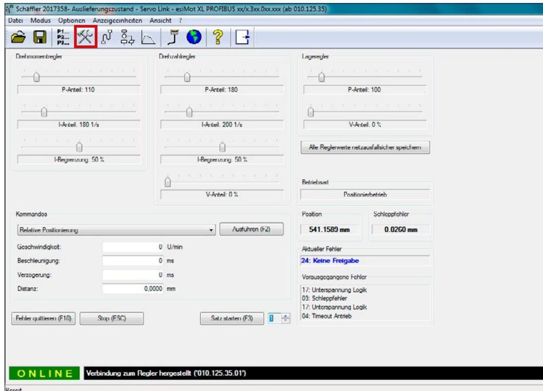
Fig. 24: Parameters for the torque, speed and position controller in 'Setup'-screen
