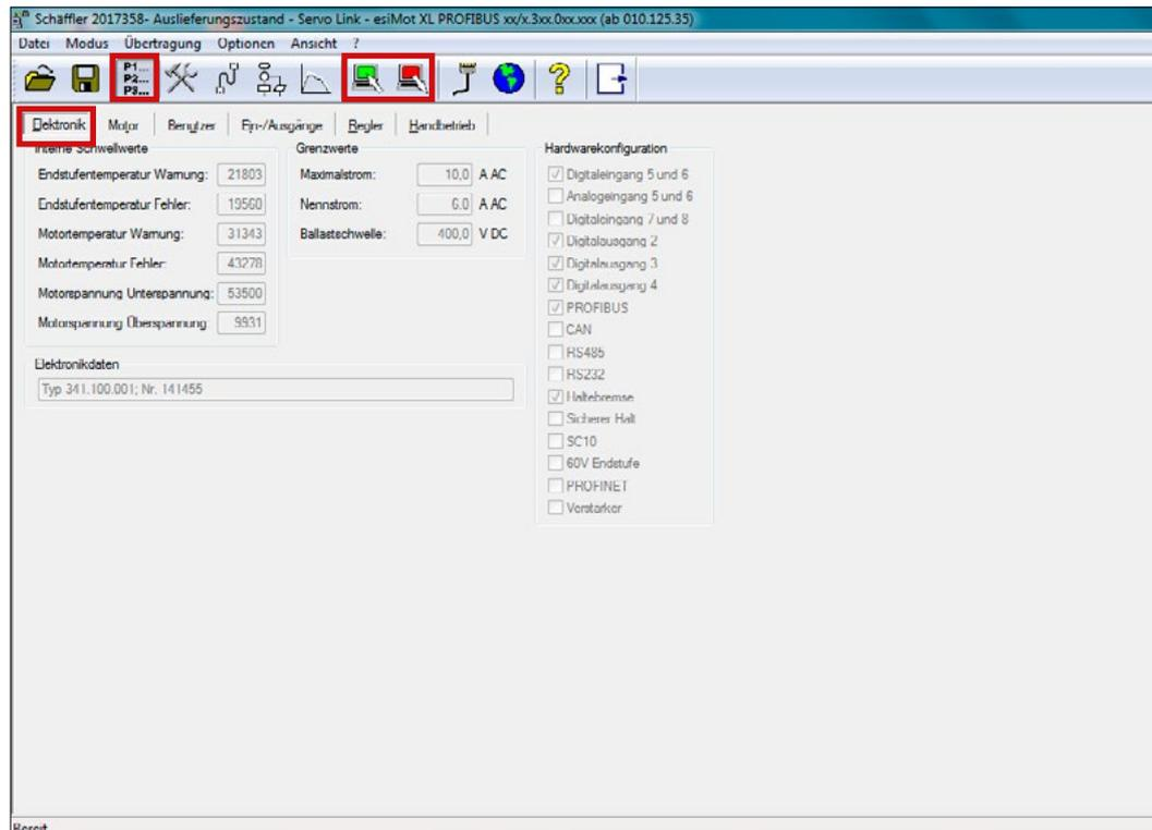
**Fig. 18:** 'Electronic'-tab in 'Parameter'-screen - parameter download to PC (green) and upload to motor control (red)
