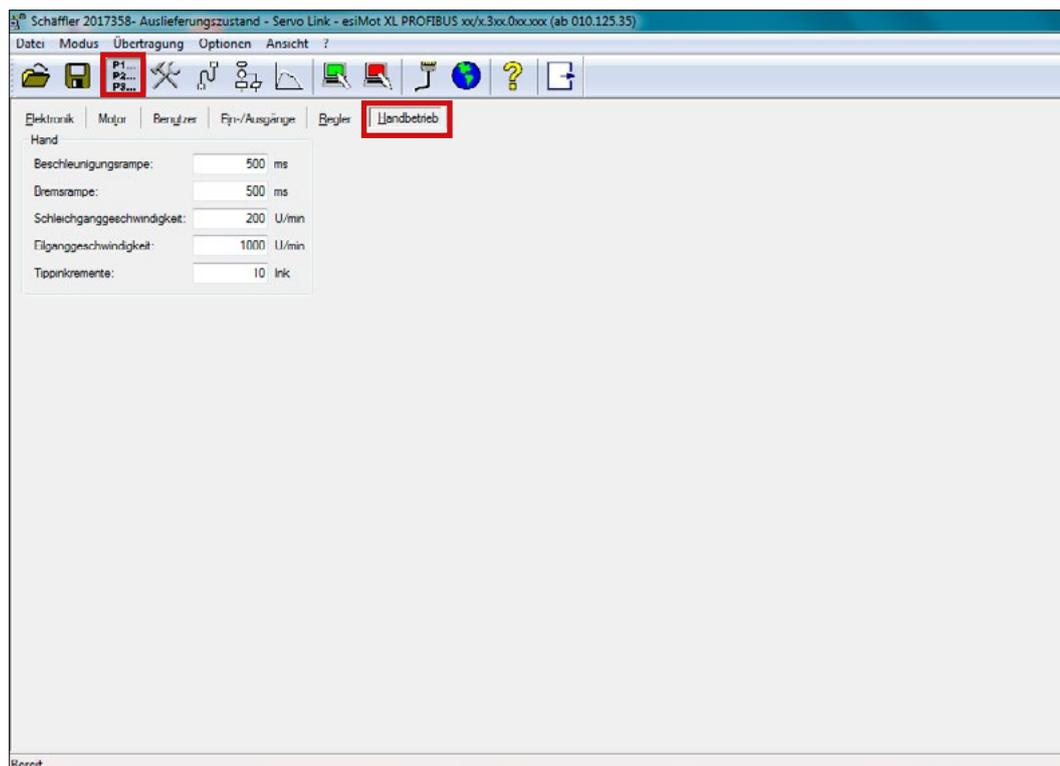
Fig. 23: 'Jog mod'-tab in 'Parameter'-screen
