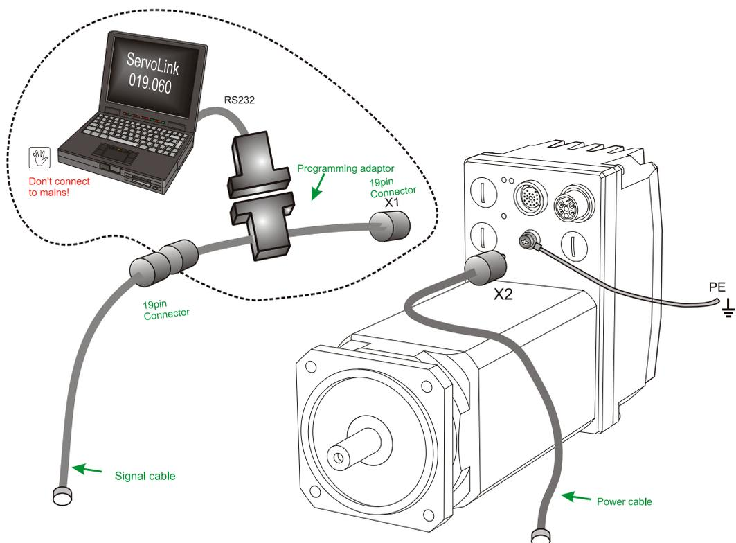
**Fig. 6:** Programming set installation
